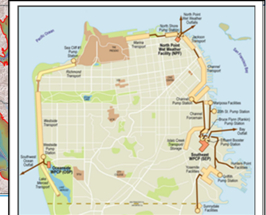
San Francisco combined sewer system transport and storage boxes (from San Francisco 2030 Sewer System Master Plan 2011)
