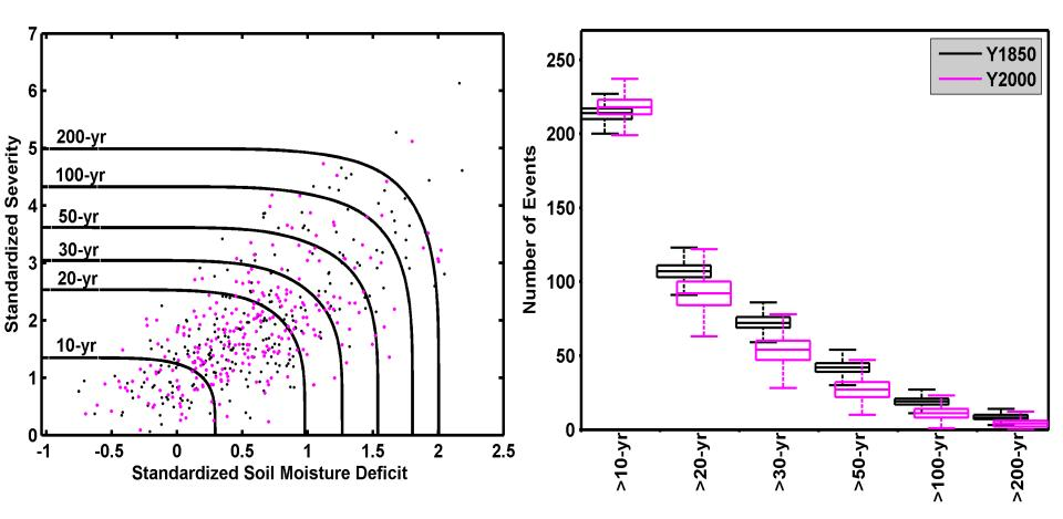
Figure 6 Joint return period of precipitation anomalies and SM anomalies at 1m using Y1850 (black dots) and Y2000 (blue dots); joint contour is based on Y1850
