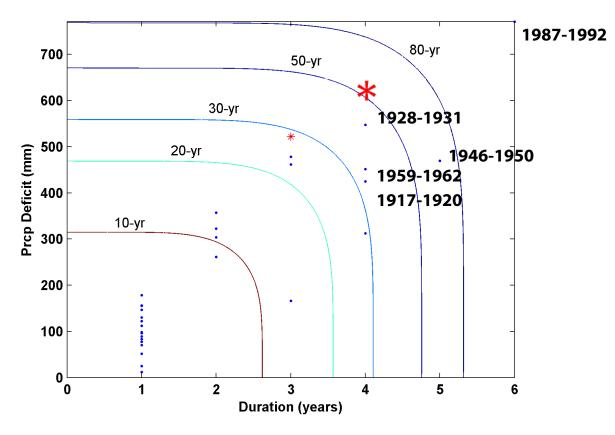
Figure 3 Joint return period of CA drought duration and severity
