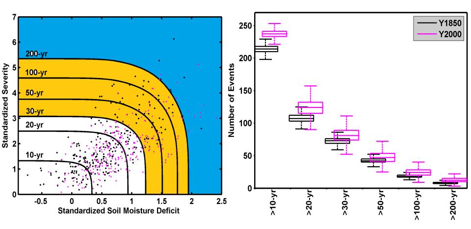
Figure 5 Joint return period of precipitation anomalies and SM anomalies at 10cm using Y1850 (black dots) and Y2000 (blue dots); joint contour line is based on Y1850
