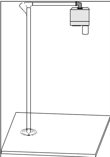
Sensor mounted on an interval stake
