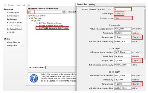
4. Click the **Wiring** tab to see how the probe is to be wired to the data logger. Click **OK** after wiring the probe.
