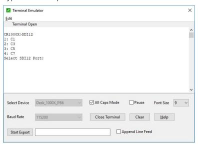
8. At the **Select SDI12 Port** prompt, type the number corresponding to the control port where the sensor is connected and press Enter. The response **Entering SDI12 Terminal** indicates that the sensor is ready to accept SDI-12 commands.
