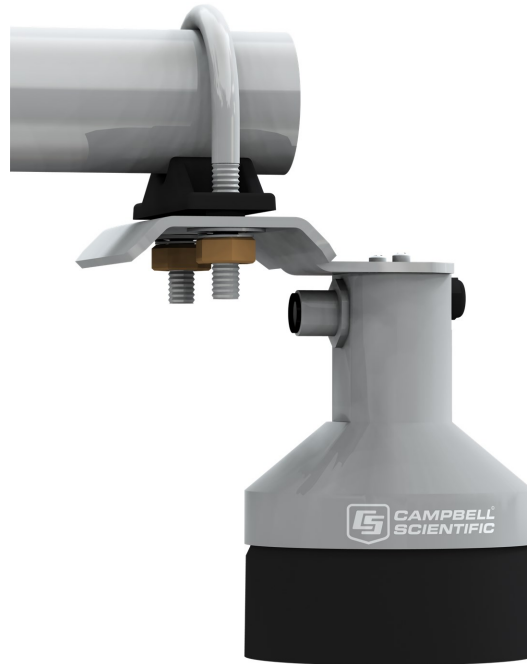
Figure 7-3. Crossarm installation using the SnowVUE 10 mounting kit
