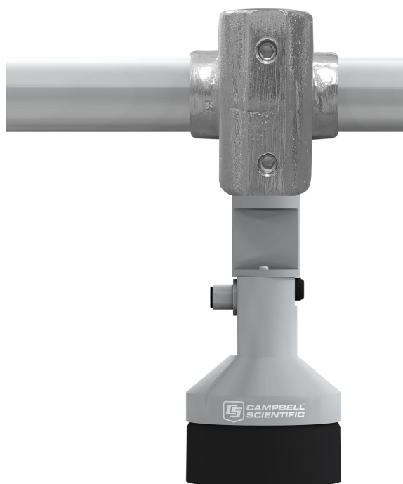
Figure 7-5. SnowVUE 10 mounted to a crossarm using the mounting stem and a 1-inch-by-1-inch Nu-Rail fitting
