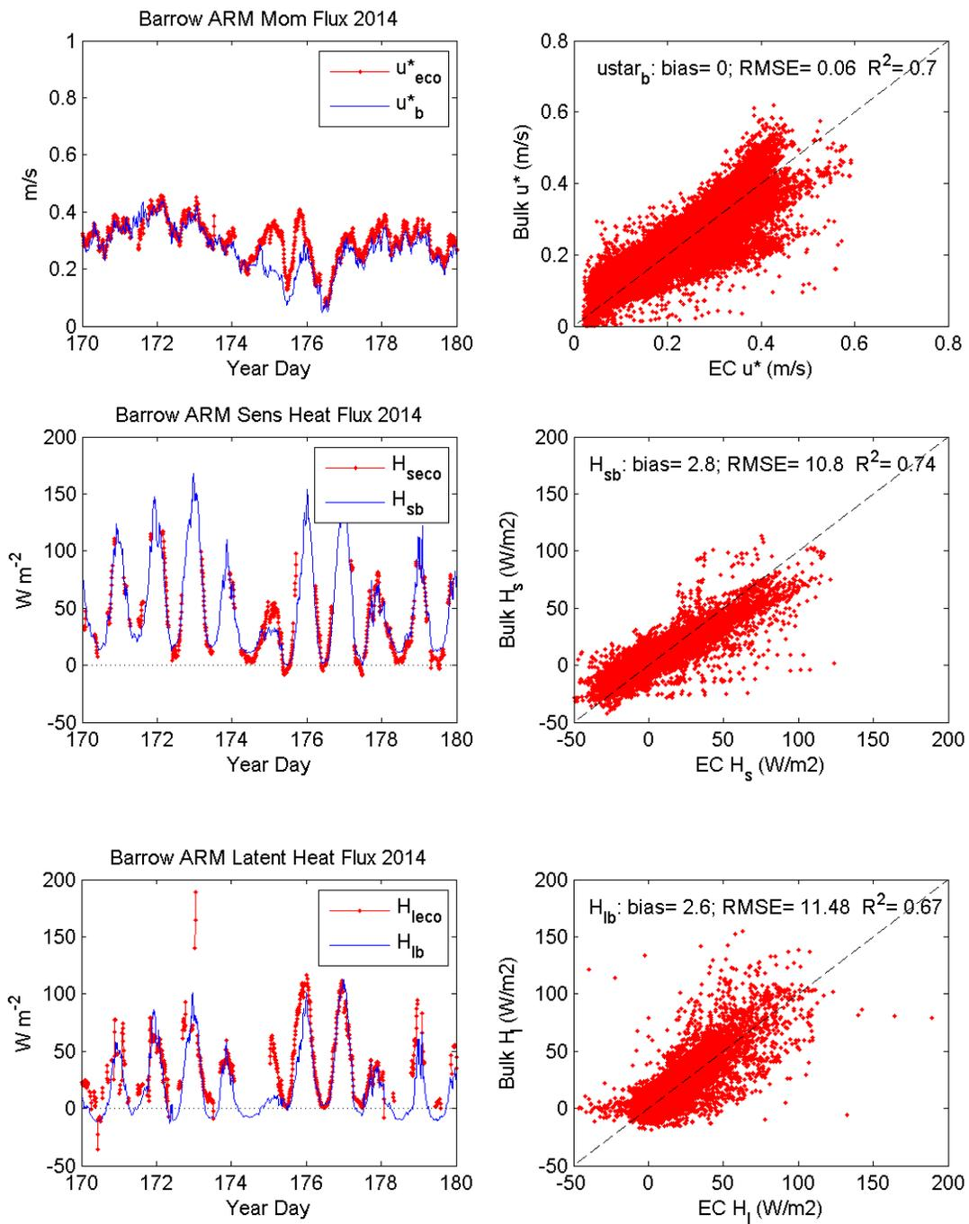
Fig. 1: Left column: Sample time series of eddy covariance (red) and bulk scheme momentum (top), sensible heat (middle), and latent heat (bottom) fluxes during 2014 at Barrow. Right column: statistical comparisons of the bulk fluxes with the eddy covariance fluxes at Barrow for the entire 2014 year.
