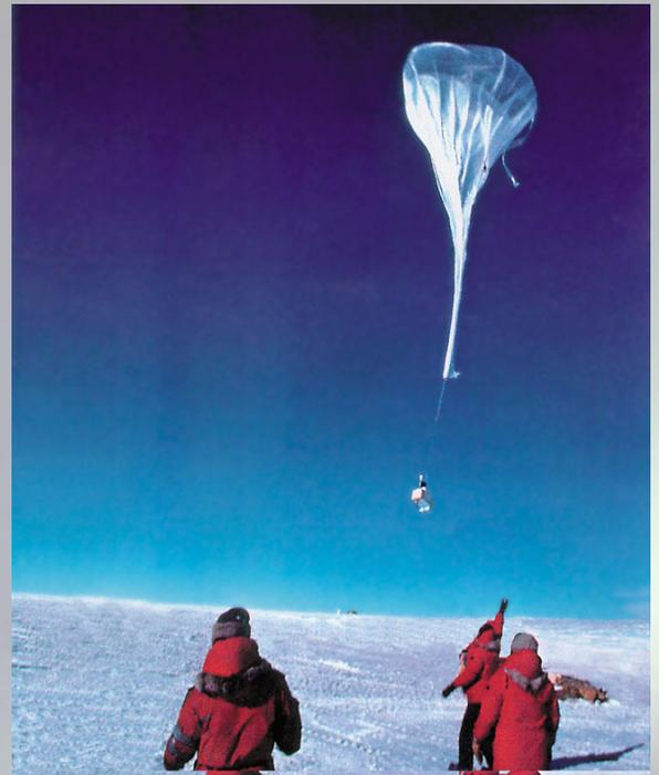
*For the NOAA team that winters over at the South Pole, one duty is launching ozone balloons and recording the data that is sent back to researchers by the instruments on the ozonesonde.*
