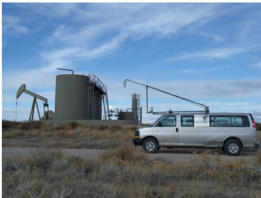
Figure 1. Mobile Lab sampling downwind of an oil well pad near Horse Pool, Uintah Basin, February 2012.
