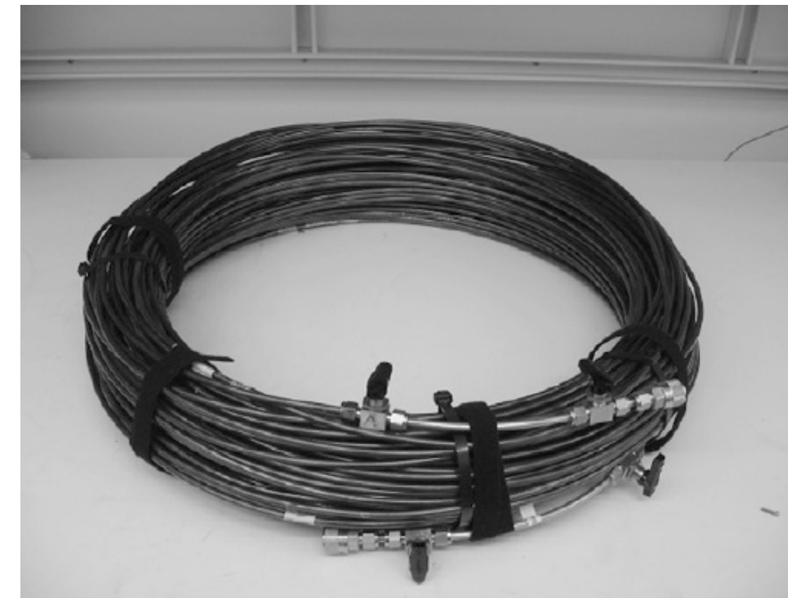
The 152 m-long AirCore, [Karion et al. 2010], More recently, [Membrive et al. 2017], [Engel et al., 2017]
