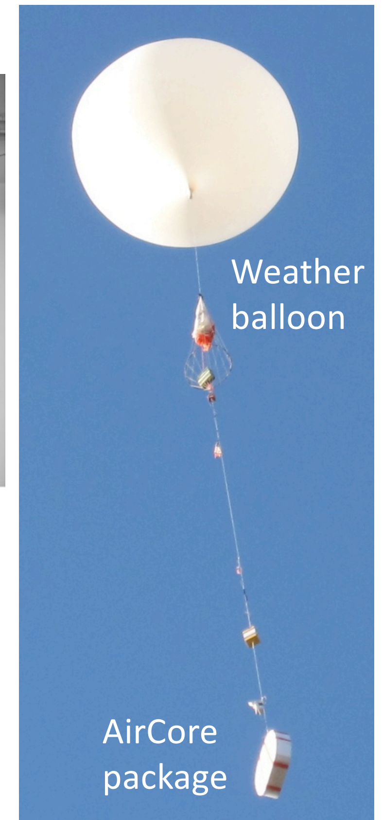
AirCore flown with a weather balloon
