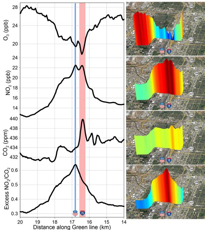
**Figure 1.** Relationships between species illustrating sources of NO<sub>2</sub> and CO<sub>2</sub> along a subsection of the TRAX line.
