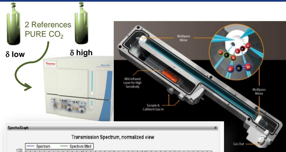
“Delta Ray uses a tunable diode laser that scans over a small spectral region in which the  $^{12}\text{CO}_2$  and  $^{13}\text{CO}_2$  isotopologues have absorption lines, fits the two corresponding peaks, determines their areas and calculate the ratio between both to provide  $\delta$ -values”.
