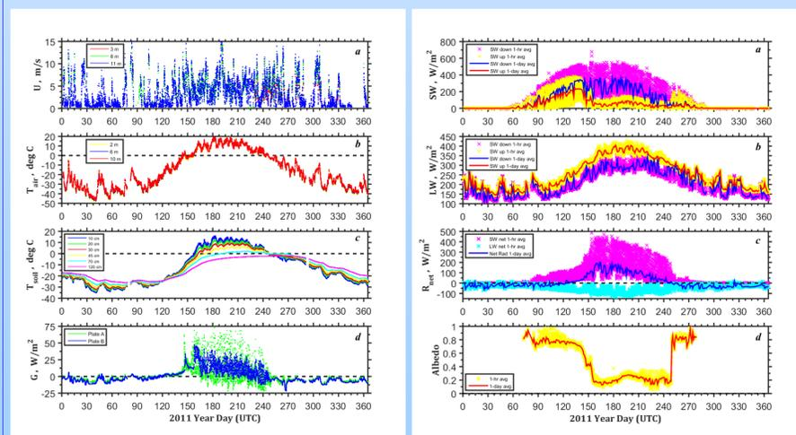
Annual cycle of (a) wind speed at 3, 8 (sonic anemometers), and 11 m (wind vane), (b) air temperature at 2, 6, and 10 m (RTD sensors), (c) soil temperature at 10, 20, 30, 45, 70, and 120 cm, and (d) soil heat flux (plates A and B) observed at Eureka in 2011. The data are based on 1-hour averaging.
