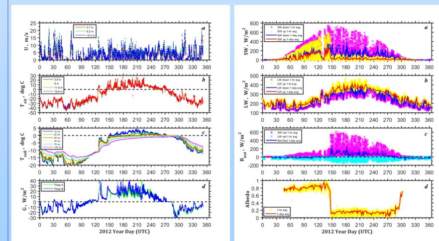
Annual cycle of (a) wind speed at 3.7, 9.2, 15.5 m (wind vanes), (b) air temperature at 3.8, 8, 11.8, 19.9 m (RTD sensors), (c) soil temperature at 10, 20, 30, 45, 70, and 120 cm, (d) soil heat flux (plates A and B) observed at Tiksi in 2012. The data are based on 1-hour averaging.
