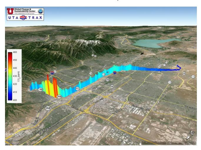
**Figure 1.** Average CO<sub>2</sub> concentrations along the Red UTA TRAX light rail route during the month-long pilot project in the summer of 2014.
