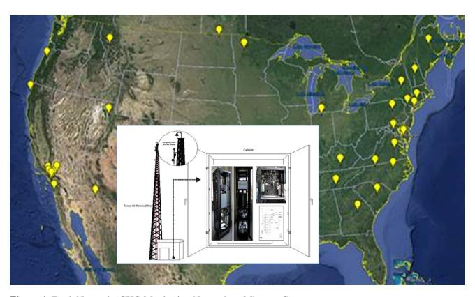
Figure 1. Earth Networks GHG Monitoring Network and System Components
