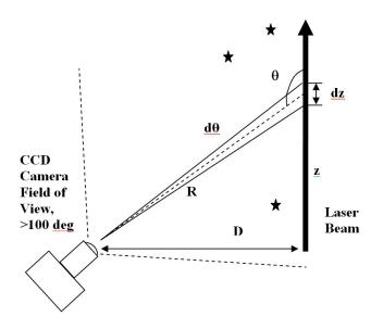
**Figure 1.** The geometry used for the CLidar technique along with three stars. The star brightness is a measured in the same images used for the CLidar aerosol profiles.
