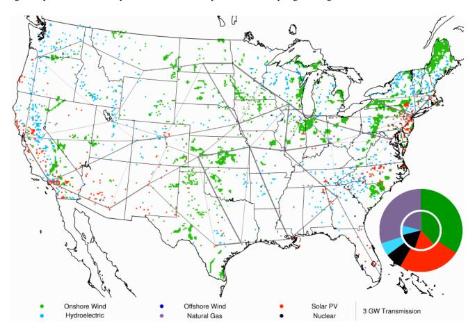
**Figure 1.** A cost-optimized single electric power system for the contiguous U.S.. The colors indicate that a model grid cell has a technology sited within it. The gray lines show the HVDC transmission network. The outer pie chart on the right represents the installed capacity by technology, while the inner pie chart shows the electric demand met by each technology. Electricity is shared across the entire U.S. along HVDC transmission lines connected to 32 nodes.
