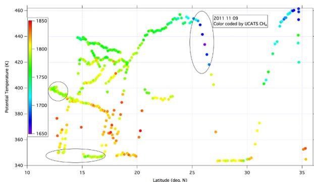
**Figure 1.** Flight track of the Global Hawk, November 9, 2011, color-coded by UCATS methane data. At 12-13°N, 390-400 K (circle), and 12-17°N, 340-350 K (horizontal oval) methane was lower (<1800 ppb) than in nearby air masses; this decrease was confirmed by concurrent flask samples. At 25°N (vertical oval), methane decreases sharply, suggesting an intrusion of high latitude air.
