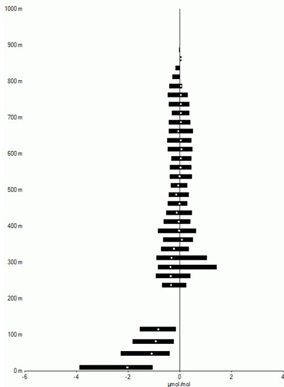
**Figure 1.** Frequency distribution (25-percentile/median/75-percentile) of the deviation between the mid-PBL CO<sub>2</sub> mole fraction and the mole fraction measured at a given elevation above the ground in summer half year (April-September).
