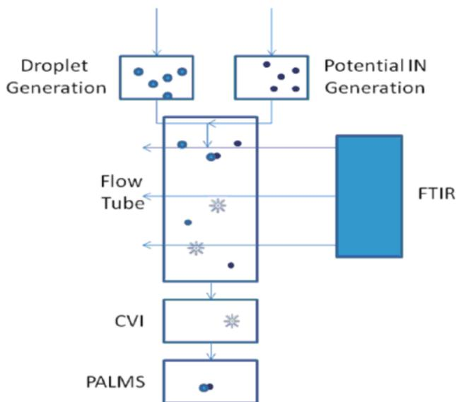
**Figure 1.** System diagram. Droplets and potential IN will be generated and equilibrated with the flow tube temperature before interacting. A Bruker FTIR spectrometer will be used to determine ice nucleation in multiple locations. A CVI will be used to separate ice crystals from unactivated aerosol particles and evaporated drop residue. The PALMS instrument will be used for ice residue analysis.
