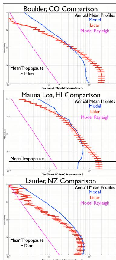
**Figure 1.** Comparison of the annual mean backscatter profile from each lidar and WACCM/CARMA (averaged at the model grid point closest to the corresponding lidar location).
