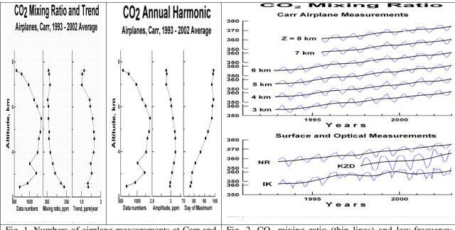
Fig. 1. Numbers of airplane measurements at Carr and average CO<sub>2</sub> mixing ratio and trends (left plot), also amplitude and day of maxima of annual harmonic (right plots) for years 1993 – 2002.
