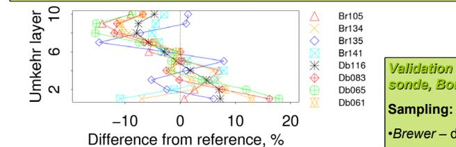
**Figure above:** Errors in the retrieved ozone for NOAA Dobson (Db) and NEUBrew (NOAA/EPA UV Brewer network) Brewer (Br) instruments in Boulder, CO, USA. Retrieval errors are associated with uncorrected OOB (out-of-band) stray light contribution in Dobson and Brewer measurements.
