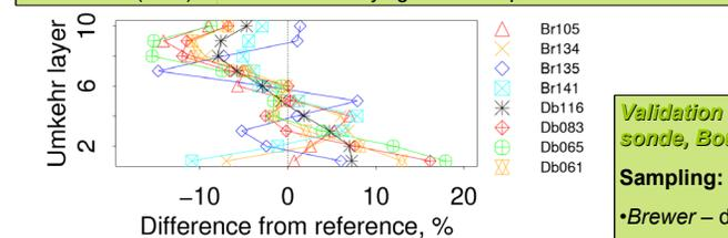
**Figure above: Errors in the retrieved ozone for NOAA Dobson (Db) and NEUBrew (NOAA/EPA UV Brewer network) Brewer (Br) instruments in Boulder, CO, USA. Retrieval errors are associated with uncorrected OOB (out-of-band) stray light contribution in Dobson and Brewer measurements.**
