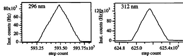
**Fig. 6** Two Hg peaks from the midnight calibration scan, taken near the end of a Hg lamp working life.
