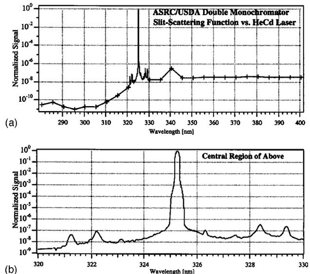
**Fig. 3** (a) Extended slit-scattering function of ASRC/USDA spectroradiometer and (b) central region of same.
