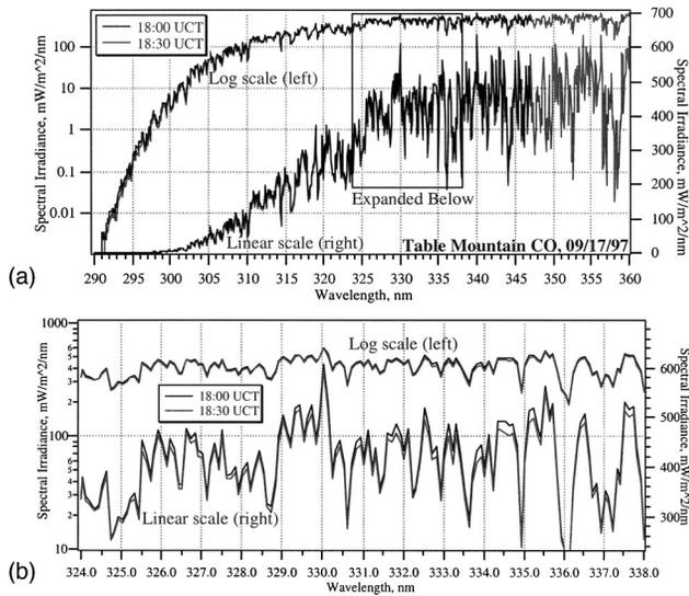
**Fig. 1** Spectra taken by the ASRC Instrument at the Table Mountain Intercomparison: (a) two sequential scans near solar noon in log and linear ordinates, and (b) expanded central region of top.
