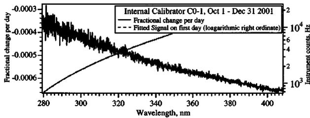
**Fig. 13** Internal calibrator C-1 trends versus wavelength in nanometers (with new fore-optic).
