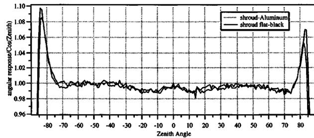
Fig. 4 Fore-optic angular response, error ratio versus cosine.
