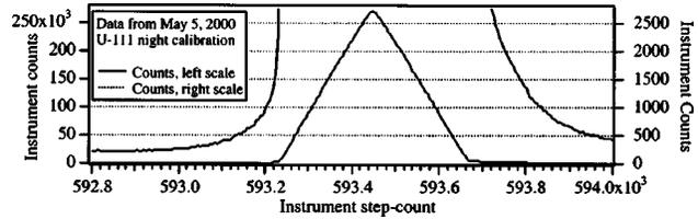
**Fig. 2** Observation of the 296.728-nm emission line of Mercury.
