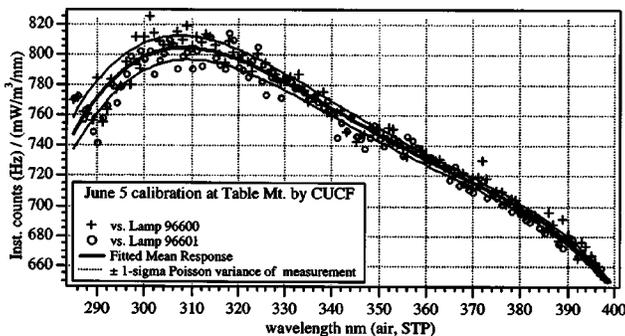
Fig. 8 Instrument responsivity from CUCF calibration.
