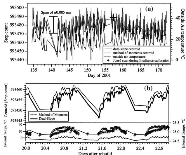
Fig. 5 (a) Time-series of 296-nm retrace centroids for May/June 2001 and (b) detail of retrace scans following lamp replacement on 29 April 2000.
