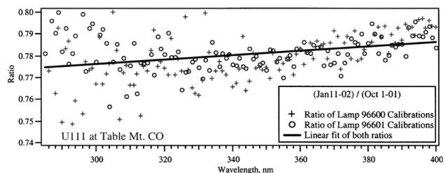
Fig. 12 Ratio of CUCF portable calibrations after the fore-optic replacement, 30 September 2001.
