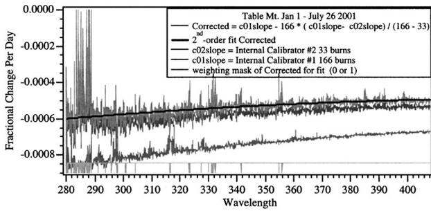
Fig. 10 Internal calibrator trends versus wavelength in nanometers.
