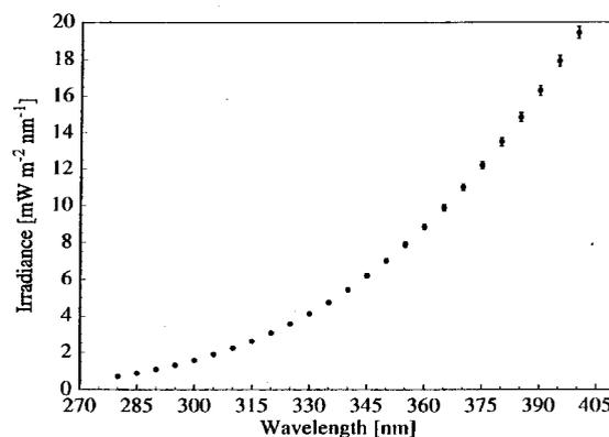
Fig. 7. Irradiance as a function of wavelength for lamp OS-27 in the horizontal position. The vertical bars indicate the expanded combined standard uncertainty (coverage factor  $k = 2$ ) of the irradiance.
