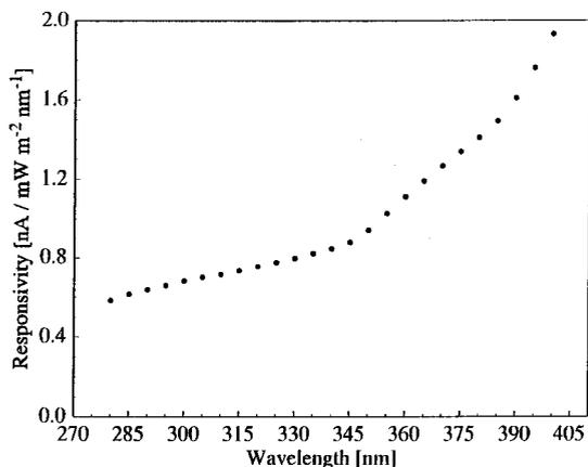
Fig. 3. Responsivity of the spectroradiometer as a function of wavelength as determined by lamp F-410 on day 2. The expanded combined standard uncertainties (coverage factor  $k = 2$ ) are comparable to the sizes of the symbols.
