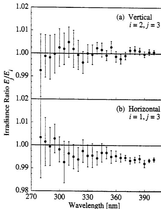
Fig. 6. Irradiance ratio  $E_j/E_i$  between days as a function of wavelength for lamp OS-27 in the (a) vertical and (b) horizontal position. The days used in the ratios are given by the indices  $i$  and  $j$ . The vertical bars indicate the expanded combined standard uncertainty (coverage factor  $k = 2$ ) of the ratios without including the uncertainty component arising from alignment of the lamps.
