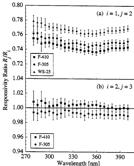
Fig. 4. Responsivity ratio  $R_j/R_i$  between days as a function of wavelength for the indicated lamps. The days used in the ratios are given by the indices  $i$  and  $j$ . The vertical bars indicate the expanded combined standard uncertainty (coverage factor  $k = 2$ ) of the ratios.
