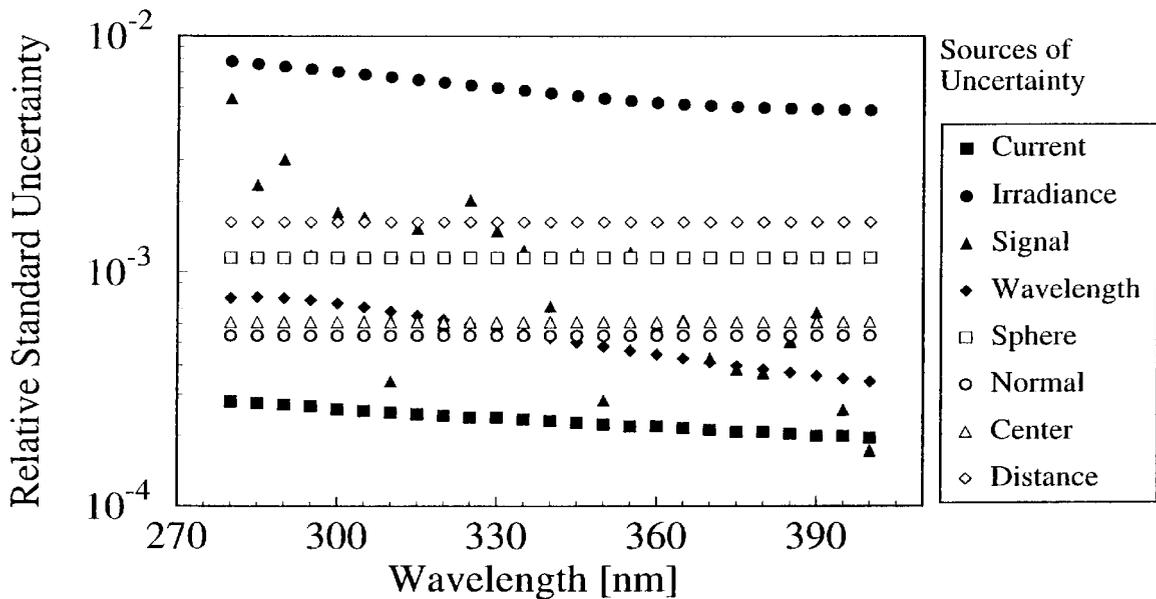
**Fig. 2.** Relative standard uncertainty components of irradiance as a function of wavelength from the indicated sources. These sources are the current through the lamp, irradiance of the lamp, signal from the detector, wavelength accuracy of the monochromator, integrating sphere orientation, and alignment of the lamp normal to and centered on the normal of the entrance port at the specified distance.
