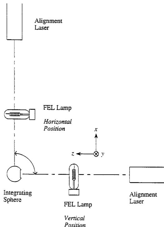
**Fig. 1.** Schematic diagram of the positions of the integrating sphere, lamps, and alignment lasers. The integrating sphere could rotate by  $90^\circ$  to view either lamp position. The position nomenclature for each lamp is indicated, along with the coordinate directions for the vertical lamp.
