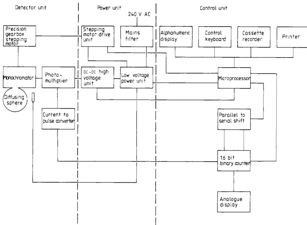
Figure 1. Schema of NRPB scanning spectral radiometer.
