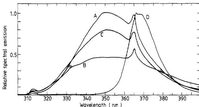
**Figure 2.** Plots of relative spectral irradiance (normalised to 351 nm) for; A, lamp with greatest emission at 351 nm; B, lamp with smallest emission at 351 nm; C, average lamp, and D, plot of relative spectral irradiance of lamp with fluorescent peak emission at 365–367 nm.
