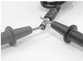
The power module output should be approximately +13V DC with no load or +9V with a load (the center pin is positive.) If the voltage is normal, then replace the RS422 adapter and test again.
