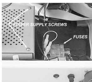
If there is still a no-power indication, then the Brewer top cover should be removed and the MAIN power supply checked to see if it feels warmer than ambient.
