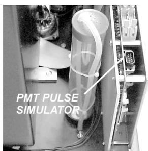
approximately 2,280,140 counts. Exit TT by pressing the Home key, turn off Brewer power, replace the PMT cable, and turn power back on.
