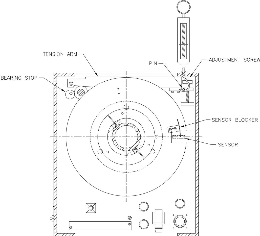
**Figure 7-1. Tracker Drive Mechanism**
