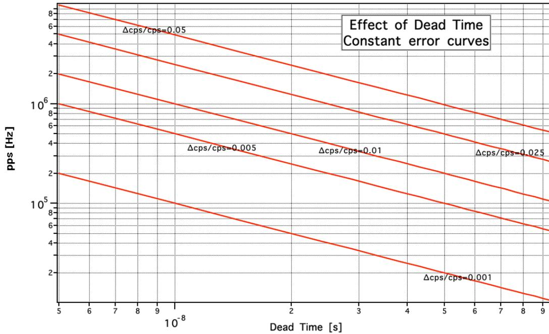
Figure 4. Effect of dead time: constant error curves.
