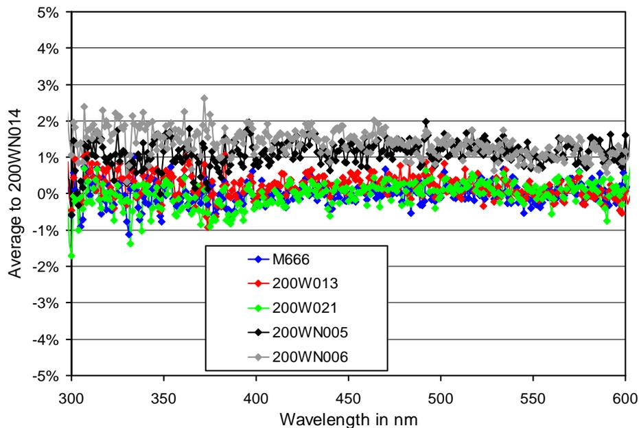
**Figure 3.1.** Comparison of South Pole lamps M-666, 200W021, 200W013, 200WN005 and 200WN006 with traveling standard 200WN014 on 24 and 25 January 2018.
