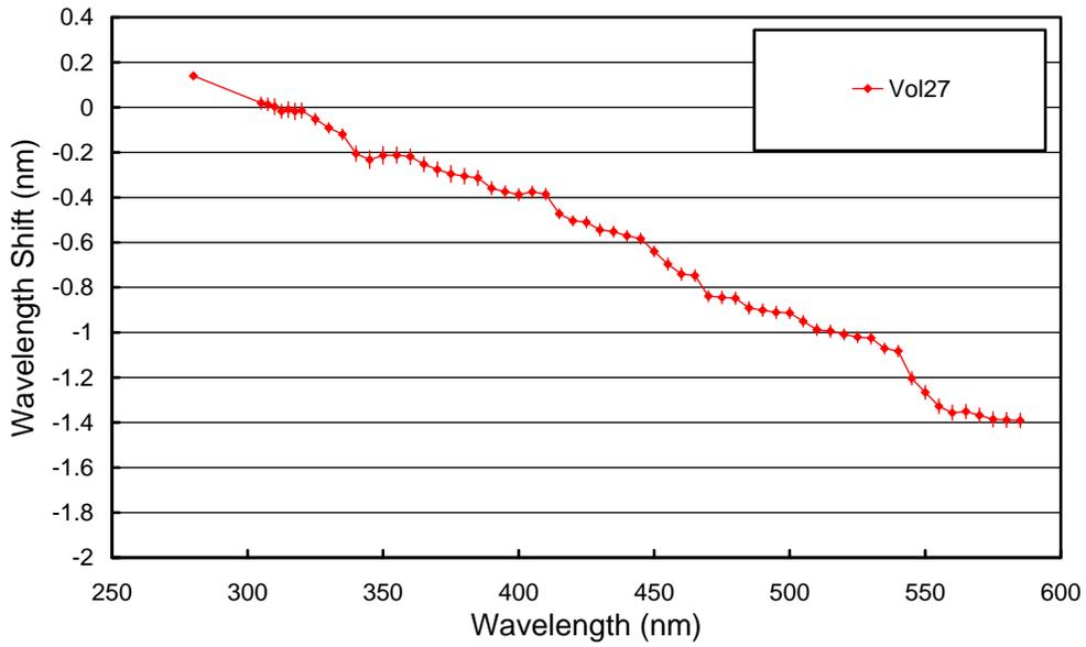
Figure 3.4. Monochromator non-linearity correction function.
