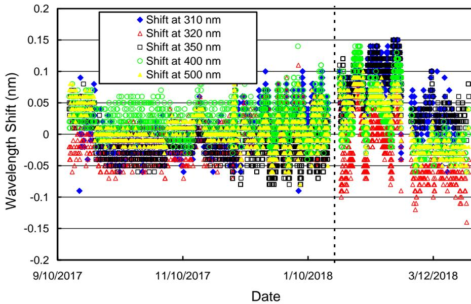
Figure 3.5. Wavelength accuracy check of *Version 0* data at five wavelengths by means of Fraunhofer-line correlation. The vertical broken line indicates the time of the site visit.
