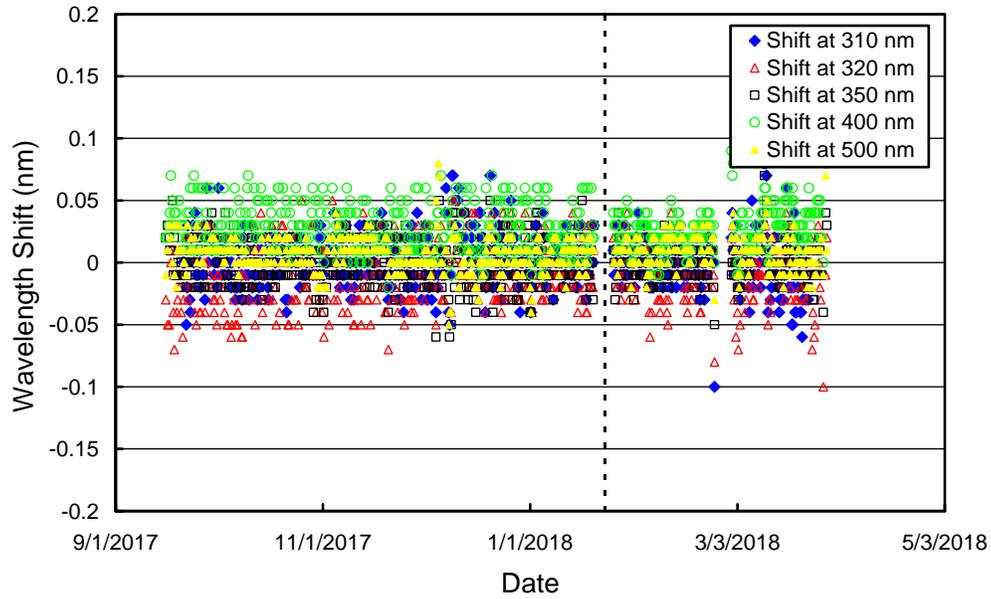
**Figure 3.6.** Wavelength accuracy check of *Version 2* data at five wavelengths by means of Fraunhofer-line correlation. The vertical broken line indicates the time of the site visit.
