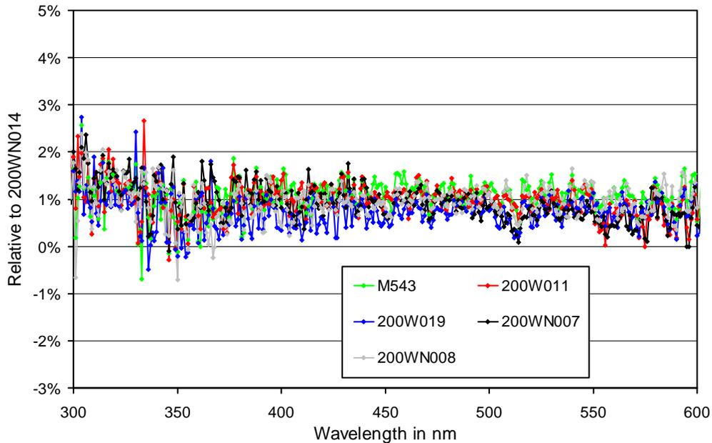
**Figure 1.** Comparison of McMurdo on-site standards M-543, 200W011, 200W019, 200WN007 and 200WN008 with traveling standard 200WN014 using absolute scans performed between 1/31/2018 and 2/4/2018.
