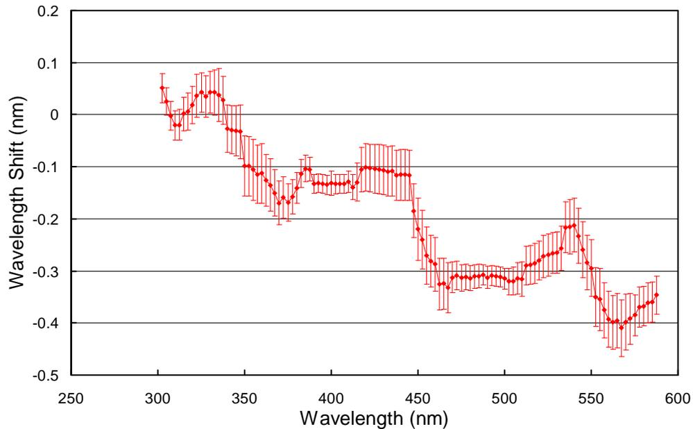
**Figure 5.** Monochromator non-linearity correction function for the Volume 27 period. Error bars indicate the  $1\sigma$ -variation.
