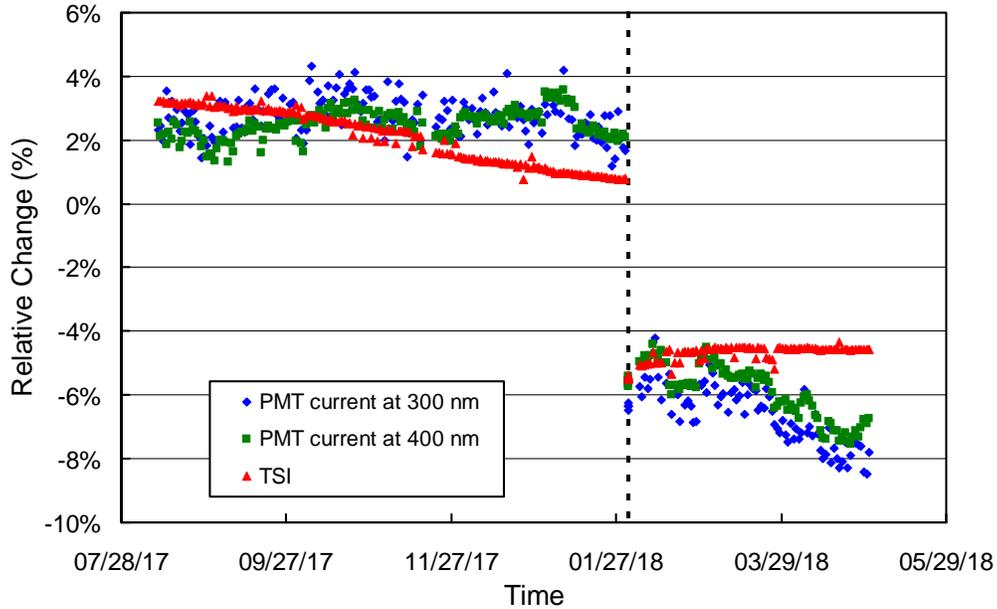
**Figure 2.** Measurements of the SUV-100’s TSI sensor and PMT currents at 300 and 400 nm. Data are shown as relative change and normalized to the average of the entire period. The broken vertical line indicates the time when the internal lamp was changed.
