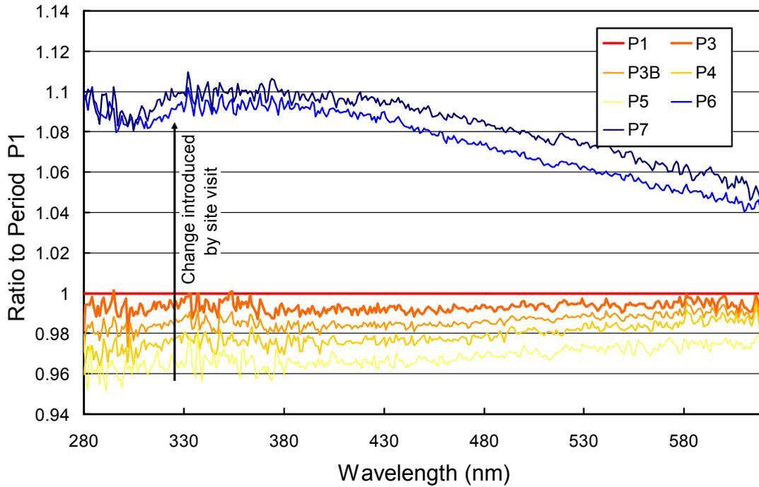
**Figure 3.** Ratios of spectral irradiance assigned to the internal reference lamp during Periods P3 through P7, relative to Period P1.
