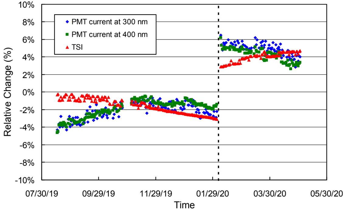
**Figure 2.** Measurements of the SUV-100’s TSI sensor and PMT currents at 300 and 400 nm. Data are shown as relative change and normalized to the average of the entire period. The broken vertical line indicates the time when the internal lamp was changed during the site visit.
