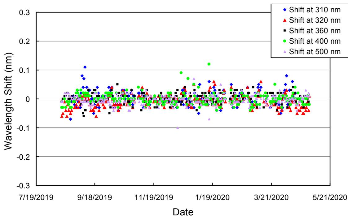
**Figure 7.** Check of the wavelength accuracy of *Version 2* data at six wavelengths by means of Fraunhofer-line correlation. The plot is based on measurements at 01:00 UT (approximate local solar noon at McMurdo).
