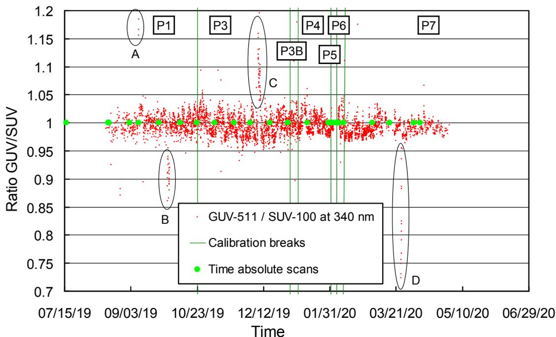
**Figure 4.** Ratio of GU-511 (340 nm channel) and SUV-100 measurements. Green vertical lines indicate times when the SUV-100 calibration was changed. The times when “absolute” calibration scans of the SUV-100 were performed are also indicated. Periods with outliers are marked with ellipses and discussed in the text.
