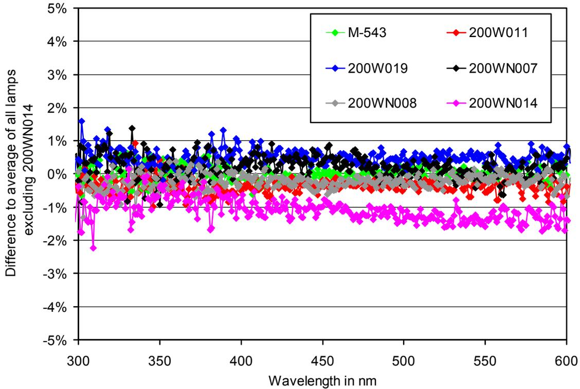
**Figure 1.** Comparison of McMurdo standards M-543, 200W011, 200W019, 200WN07, and 200WN008, plus the traveling standard 200WN014 using absolute scans performed on 2/5/20 and 2/6/20.
