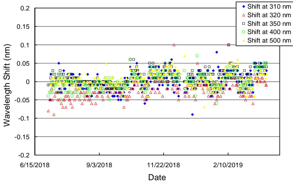
**Figure 6.** Wavelength accuracy check of the final *Version 0* data at five wavelengths by means of Fraunhofer-line correlation. Noontime measurements from every day of the year have been evaluated.
