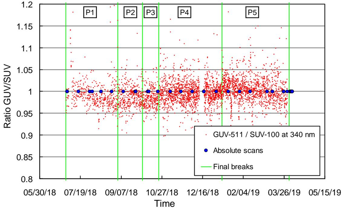
**Figure 4.** Ratio of GUV-511 measurements at 340 nm with final SUV-100 measurements. The latter were weighted with the spectral response function of the GUV-511's 340 nm channel. Narrow clusters of vertical data points are caused by snow covering the SUV-100 collector.
