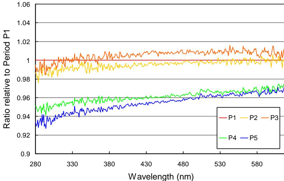
**Figure 3.** Ratios of spectral irradiance assigned to the internal reference lamp for periods P1 – P5 relative to Period P1.
