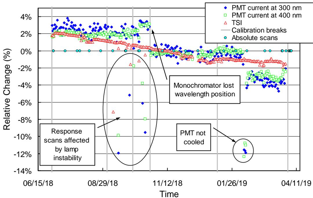
**Figure 2.** Time-series of PMT current at 300 and 400 nm, and TSI signal. All data were extracted from measurements of the internal irradiance standard and are normalized to their average. Calibration break points (Table 1) and times of absolute scans are also indicated.
