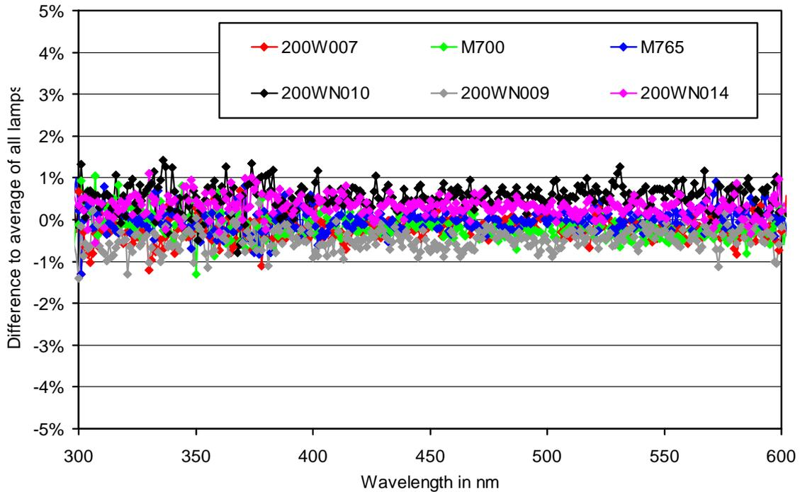
**Figure 1.** Comparison of the calibration of on-site standards 200W007, M700, and M765 with long-term standards 200WN009 and 200WN010, and the traveling standard 200WN014 on 3/25/2019.
