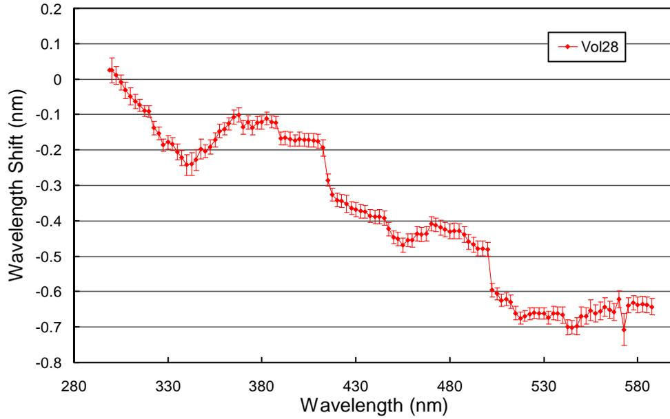
**Figure 5.** Monochromator mapping function. Error bars indicate  $1\text{-}\sigma$  variation.
