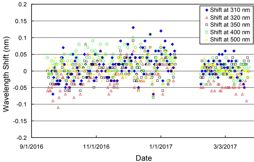
Figure 3.5. Wavelength accuracy check of Version 0 data at five wavelengths by means of Fraunhofer-line correlation.
