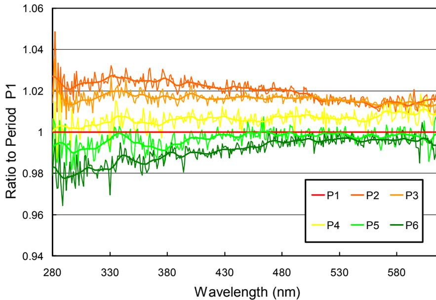
**Figure 3.3.** Ratios of spectral irradiance assigned to the internal lamp relative to Period P1 (09/14/16 – 11/17/16). Thick lines indicate the smoothed datasets.
