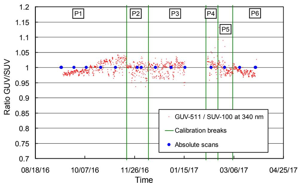
**Figure 3.2.** Ratio of GUV-541 S/N 29239 measurements (340 nm channel) with SUV-100 measurements. SUV-100 data were weighted with the spectral response function of this GUV channel. The vertical green lines indicate times when the calibration applied to SUV-100 data was changed (see also Table 3.1).
