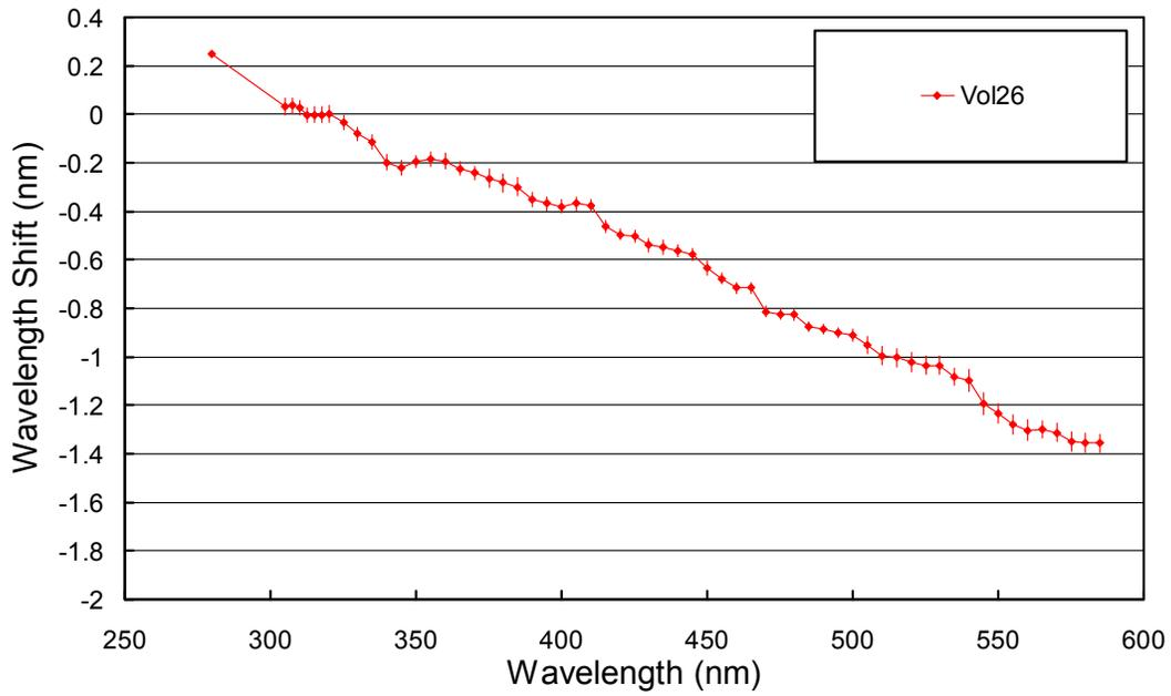
Figure 3.4. Monochromator non-linearity correction function.
