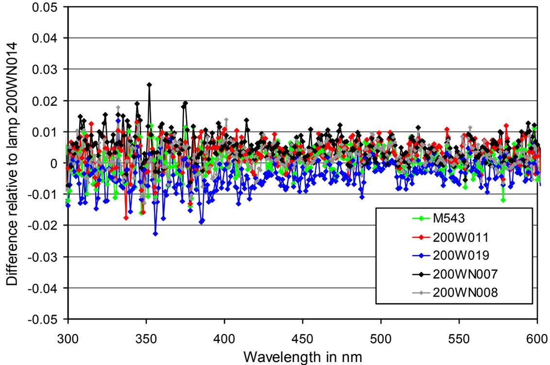
**Figure 1.** Comparison of McMurdo on-site standards M543, 200W011, 200W019, 200WN007, and 200WN008 with the traveling standard 200W014 using absolute scans performed at the start of the February 2016 site visit.
