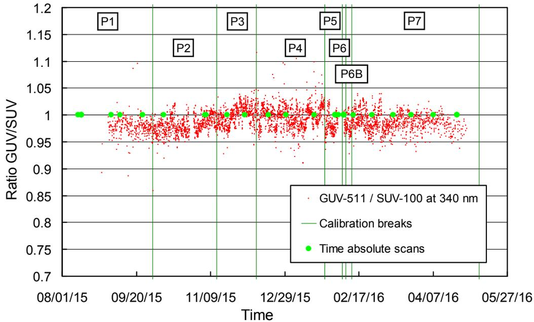
**Figure 3.** Ratio of GUV-511 (340 nm channel) and SUV-100 measurements. Green vertical lines indicate times when the SUV-100 calibration was changed. The times when “absolute” calibration scans of the SUV were performed are also indicated.
