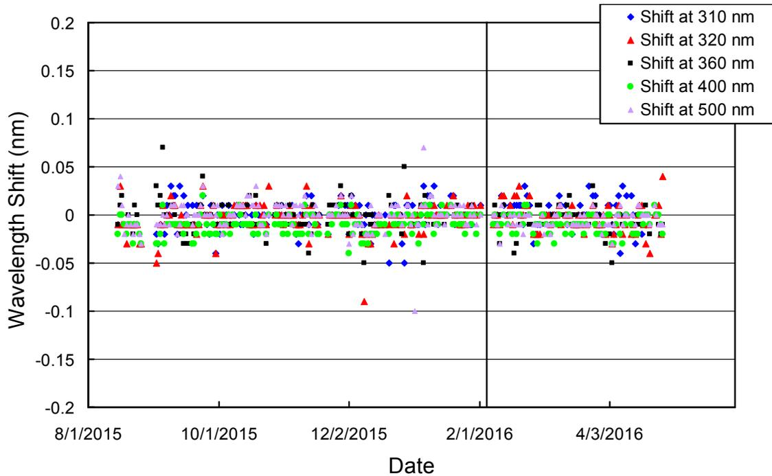
**Figure 7.** Check of the wavelength accuracy of final Version 2 data at six wavelengths by means of Fraunhofer-line correlation. The plot is based on daily measurements at noon. The vertical line indicates the time of the site visit.
