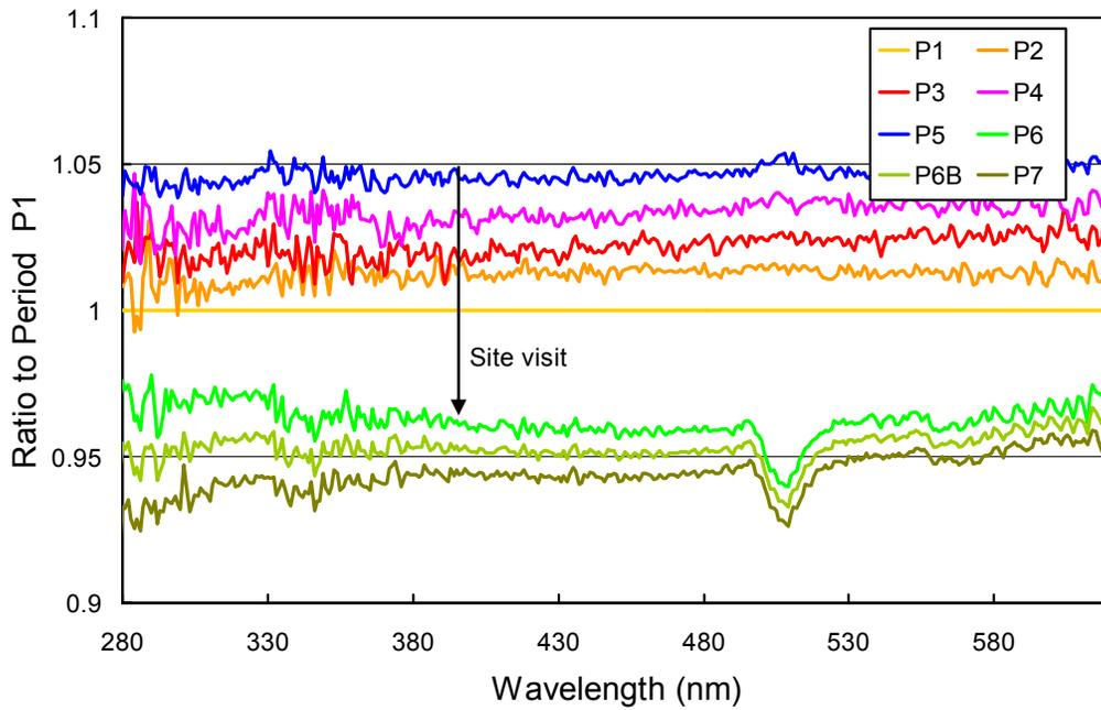
**Figure 2.** Ratios of spectral irradiance assigned to the internal reference lamp during Periods P2 through P7, relative to Period P1. The large change in the ratio between Periods P5 and P6 is caused by service performed during the February 2016 site visit when the instrument was disassembled, cleaned, and reassembled.
