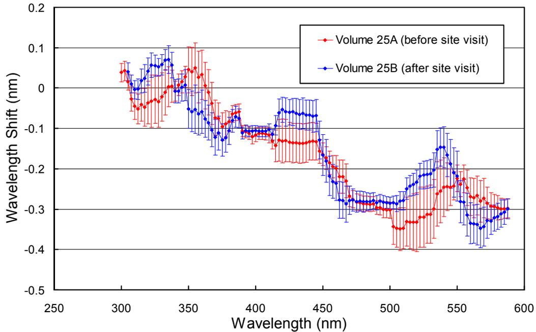
**Figure 5.** Monochromator non-linearity correction functions for the Volume 25 period. Error bars indicate the  $1\sigma$ -variation.
