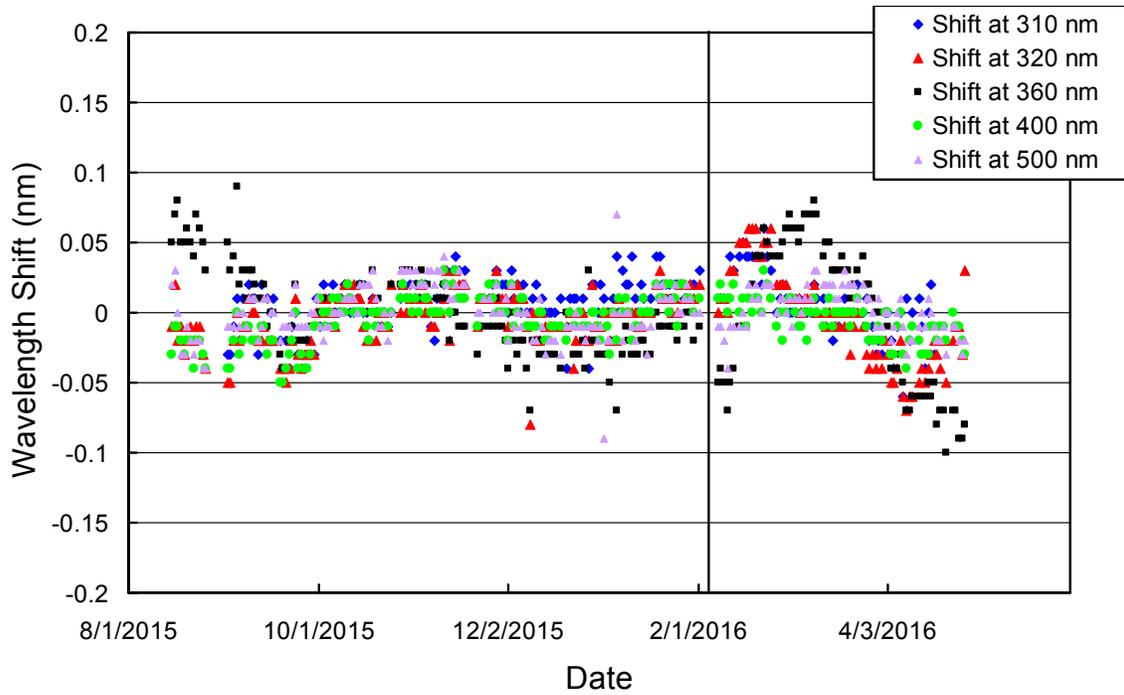
**Figure 6.** Check of the wavelength accuracy of final Version 0 data at six wavelengths by means of Fraunhofer-line correlation. The plot is based on daily measurements at noon. The vertical line indicates the time of the site visit.
