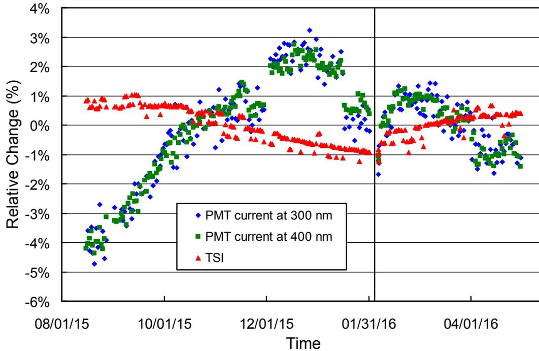
**Figure 2.** Measurements of the SUV-100's TSI sensor and PMT currents at 300 and 400 nm. Data are shown as relative change. Data measured before and after the time of the site visit (vertical line) are normalized separately.
