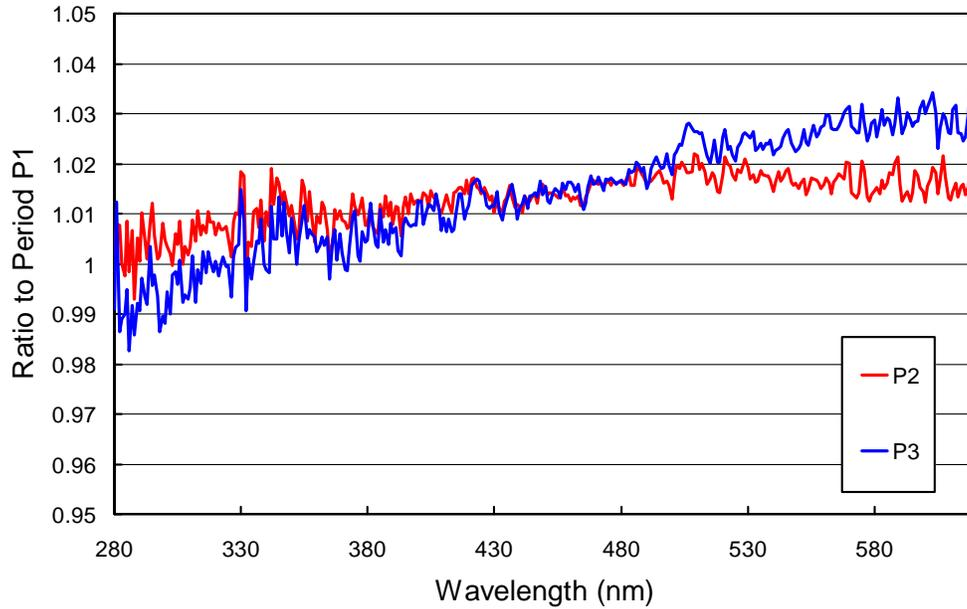
**Figure 2.** Ratios of spectral irradiance assigned to the internal reference lamp during periods P2 and P3, relative to Period P1. Changes from period to period are smaller than 2%.
