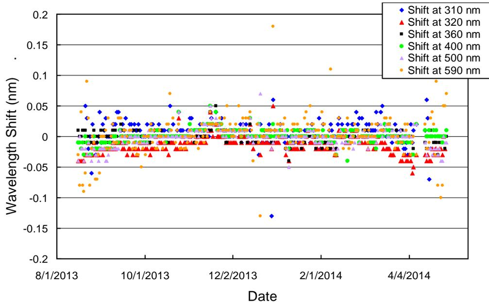
**Figure 6.** Check of the wavelength accuracy of final Version 0 data at six wavelengths by means of Fraunhofer-line correlation. The plot is based on daily measurements at noon.
