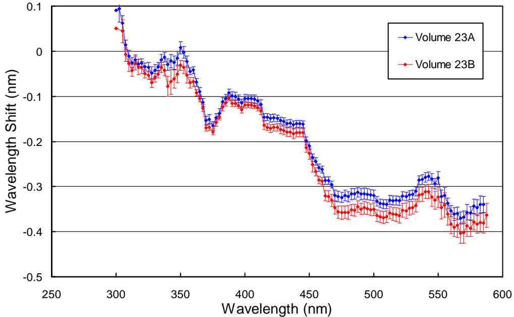
**Figure 5.** Monochromator non-linearity correction functions for the Volume 23 period. Error bars indicate the  $1\sigma$ -variation. The function labeled “Volume 23A” was applied to solar data of the period 6/22/13 – 2/10/14 and the function labeled “Volume 22B” was applied solar data of the period 2/11/14 – 6/21/14.
