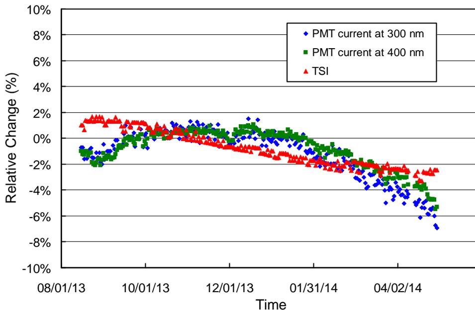
**Figure 1.** Measurements of the SUV-100’s TSI sensor and PMT currents at 300 and 400 nm. Data are shown as relative change, normalized to the average of all measurements.
