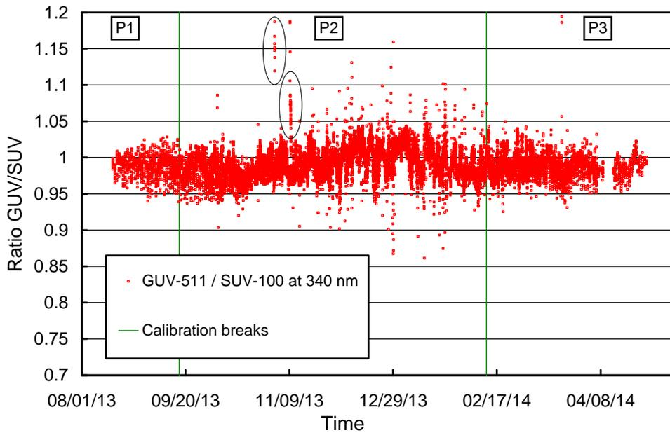
**Figure 3.** Ratio of GUV-511 (340 nm channel) and SUV-100 measurements. Green vertical lines indicate times when the SUV-100 calibration was changed. Circles indicate times when the ratio of GUV and SUV measurements was abnormally large, likely due to snow accumulation on the SUV collector. The affected scans were marked in the Version 2 data set.
