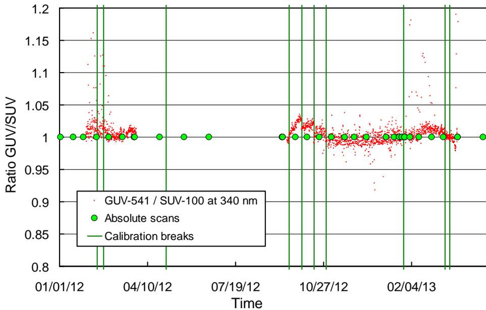
**Figure 5.3.4c.** Ratio of GUV-541 #29239 measurements (340 nm channel) with SUV-100 measurements that were weighted with the spectral response function of this channel. The plot includes the period when the refurbished GUV-541 #29239 was installed. The vertical lines indicate a change in the SUV-100 calibration applied to solar data (see Table 5.3.2). Times when absolute scans with standard lamps were executed are indicated by green circles.
