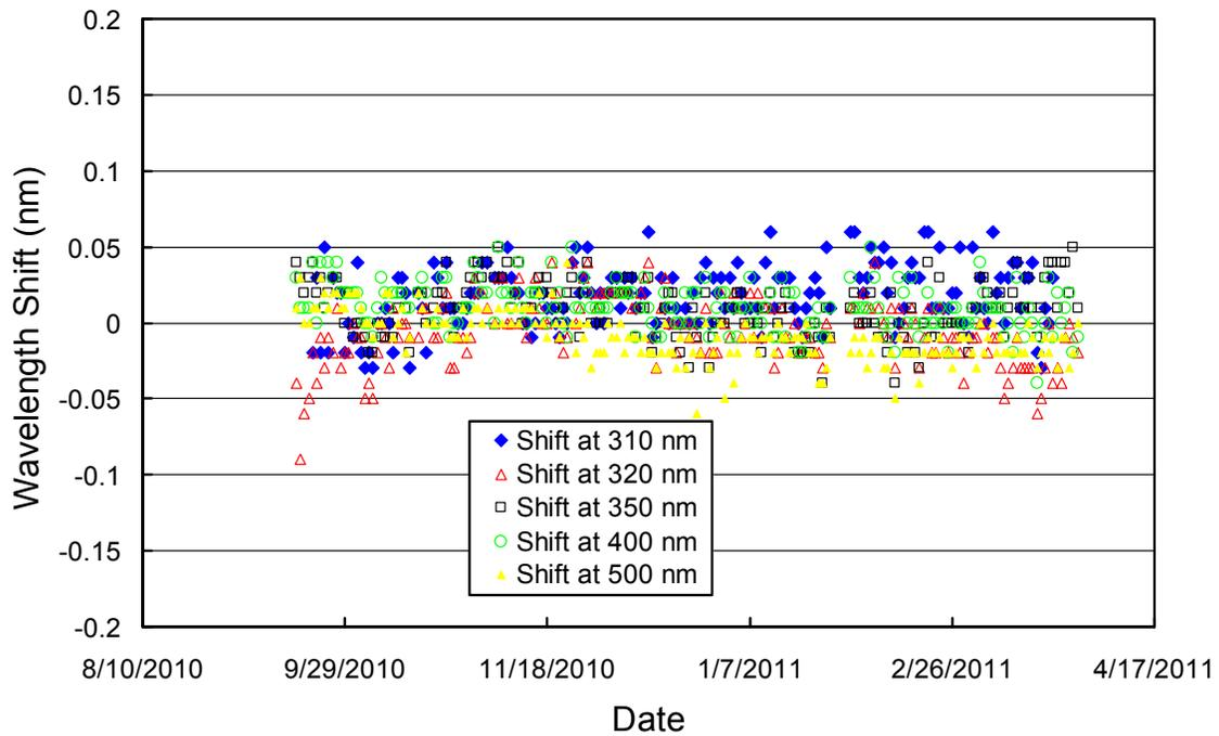
Figure 5.3.5. Wavelength accuracy check of final data at four wavelengths by means of Fraunhofer-line correlation. Measurement performed at 00:00 UT were evaluated for each day of the season. No data exist during Polar Night.
