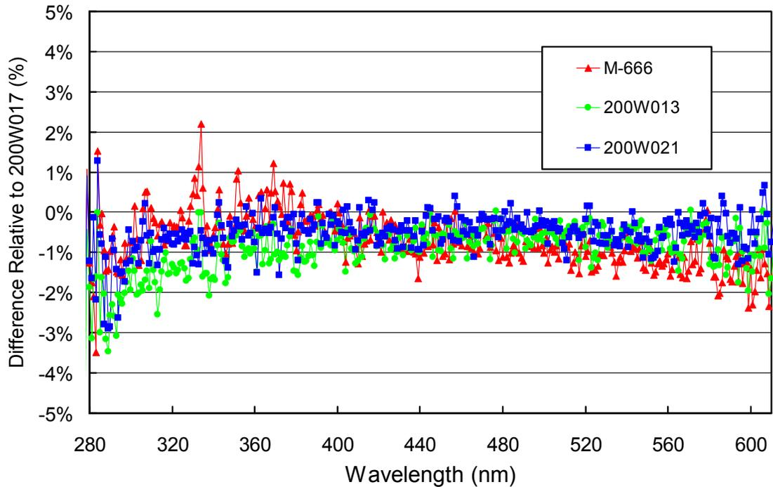
**Figure 5.3.1.** Comparison of South Pole lamps M-666, 200W021, and 200W013 with BSI traveling standard 200W017 on 1/27/2011.
