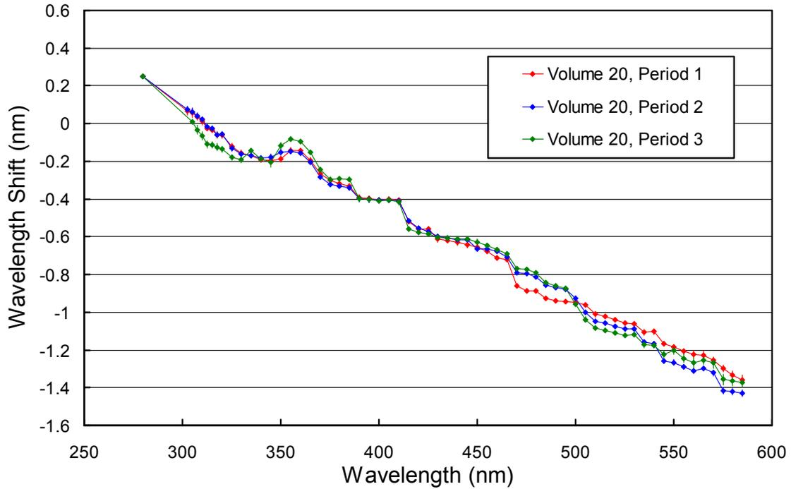
Figure 5.3.4. Monochromator non-linearity correction functions for the South Pole 2010/11 season.
