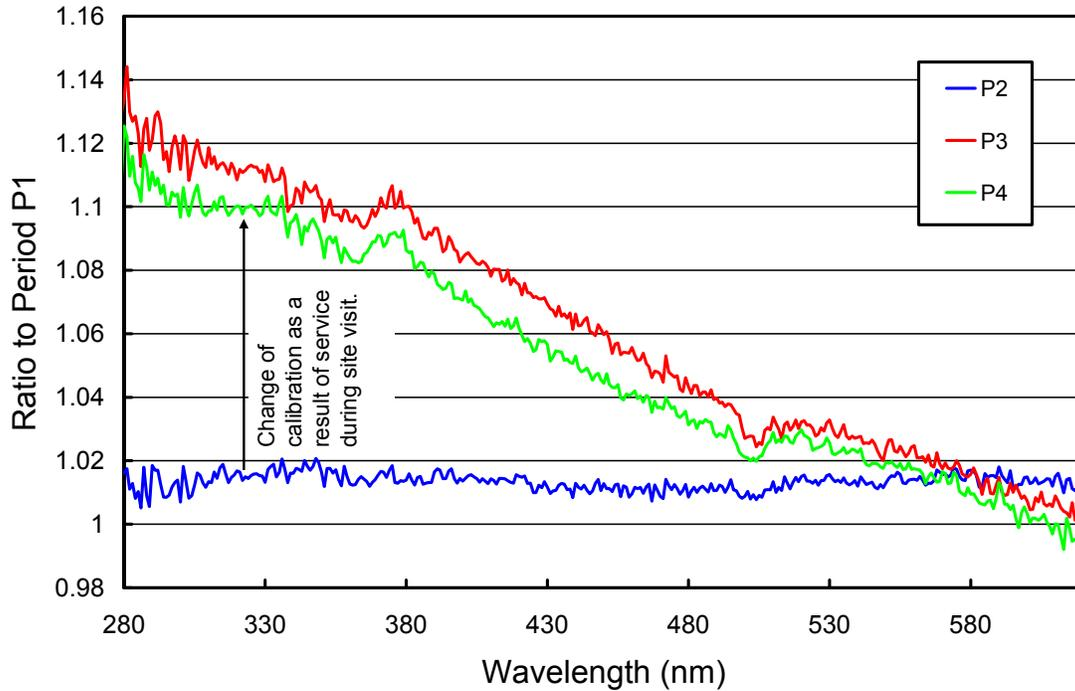
**Figure 5.3.3.** Ratios of spectral irradiance assigned to the internal lamp relative to Period P1.
