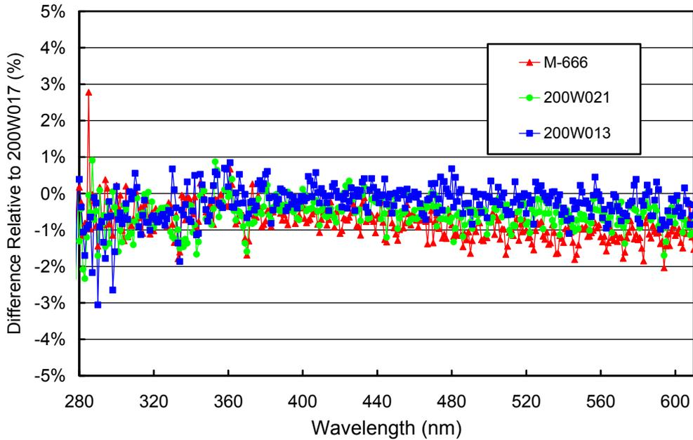
**Figure 5.3.1.** Comparison of South Pole lamps M-666, 200W021, and 200W013 with BSI traveling standard 200W017 on 2/4/2010.
