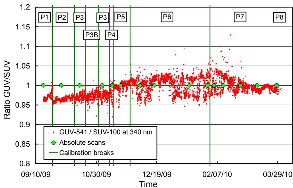
**Figure 5.3.2.** Ratio of GUV-541 measurements of its 340 nm channel with final SUV-100 measurements that were weighted with the spectral response function of this channel.
