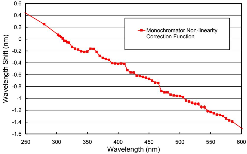
**Figure 5.3.8.** Monochromator non-linearity correction function for the South Pole 2009/10 season.
