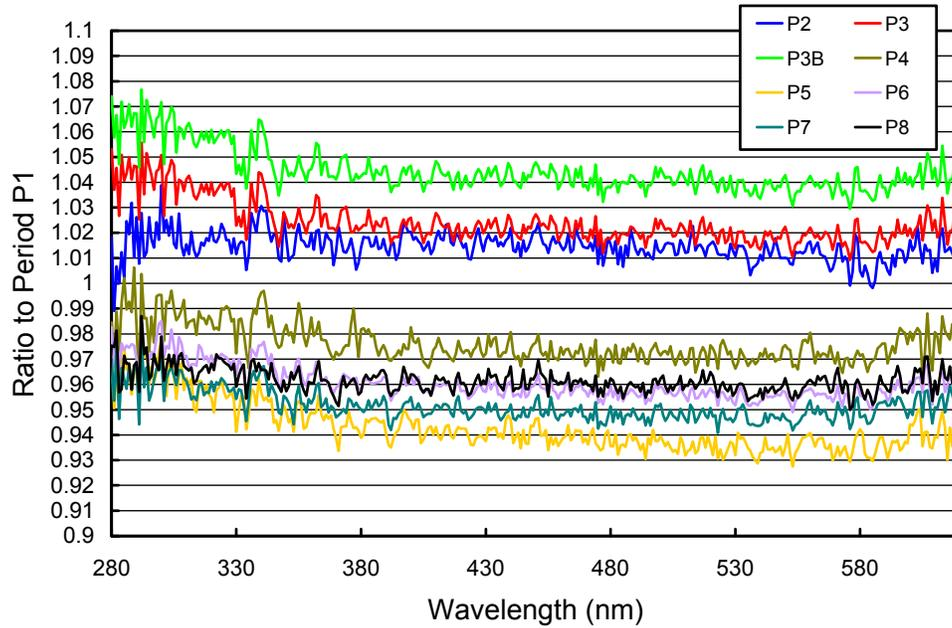
**Figure 5.3.3.** Ratios of irradiance assigned to the internal lamp relative to Period P1.
