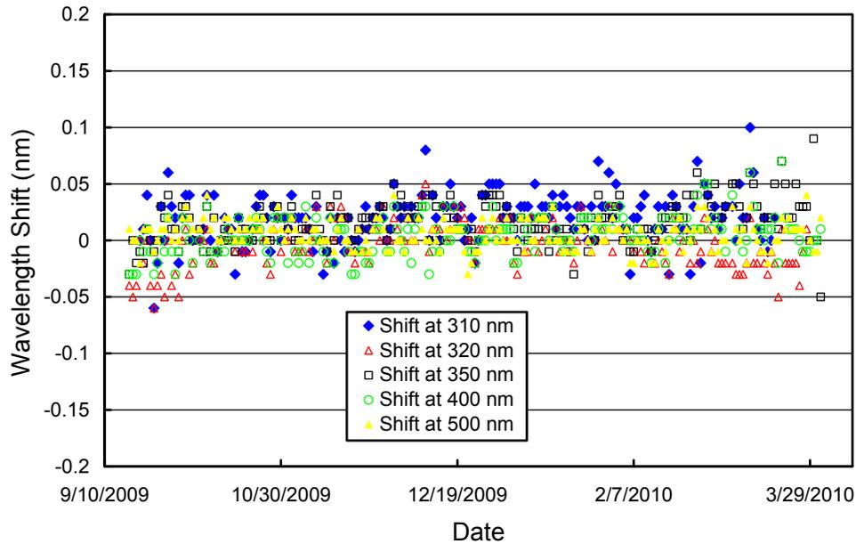
**Figure 5.3.9.** Wavelength accuracy check of final data at four wavelengths by means of Fraunhofer-line correlation. Measurement performed at 00:00 UT were evaluated for each day of the season. No data exist during Polar Night.
