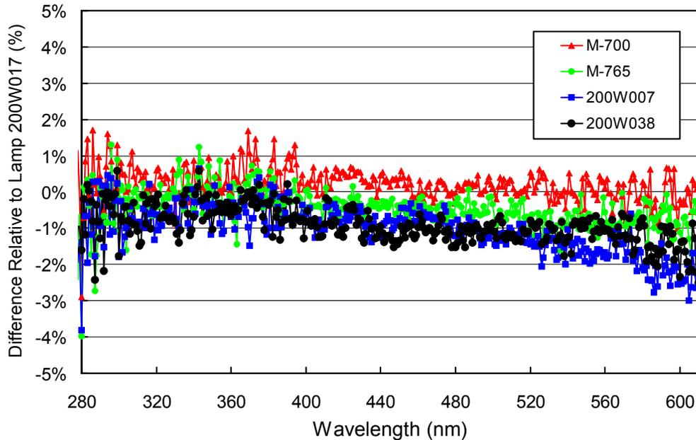
**Figure 5.2.1.** Comparison of lamps M-700, M-765, 200W007, and 200W038 with BSI traveling standard 200W017 at the beginning of the Volume 18 period. The calibration of lamp 200W017 was established by comparison with a set of four 1000-W FEL lamps that had been calibrated by NOAA's Central UV Calibration Facility (CUCF).
