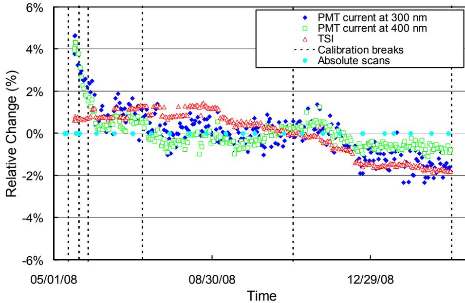
**Figure 5.2.2.** Time-series of PMT current at 300 and 400 nm, and TSI signal calculated from measurements of the internal irradiance reference. All data sets are normalized to their average values. Calibration breaks are indicated by vertical broken lines. Times of absolute scans are indicated by cyan circles.
