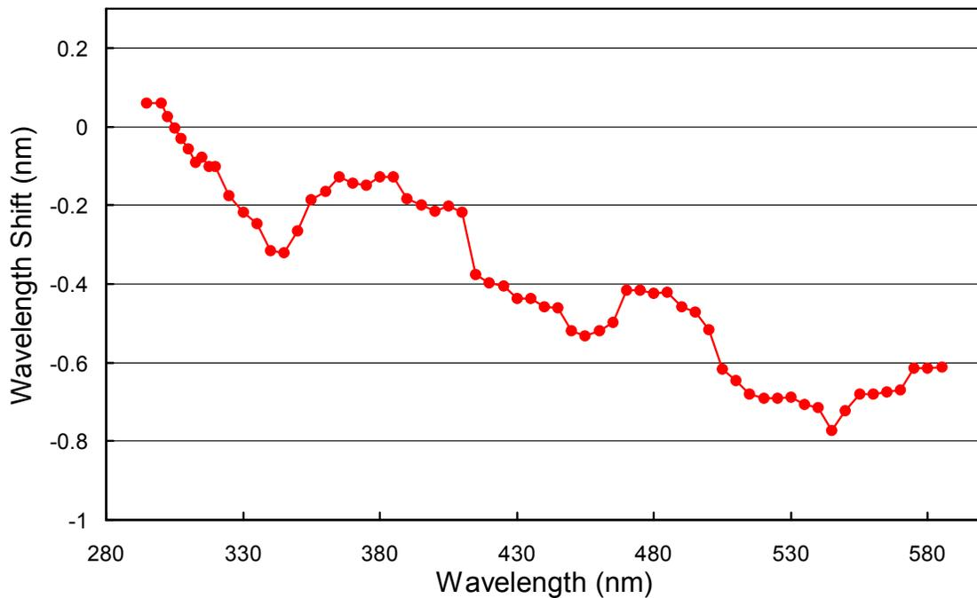
**Figure 5.2.7.** Monochromator mapping function.
