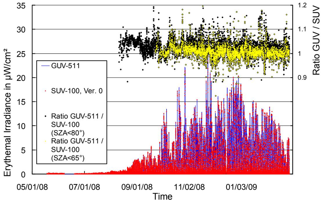
**Figure 5.2.9.** Comparison of erythemal irradiance measured by the SUV-100 spectroradiometer and the GUV-511 radiometer of the Volume 18 period. The ratio was filtered for measurements performed at solar zenith angles smaller than  $80^\circ$  (black markers) and  $65^\circ$  (yellow markers).
