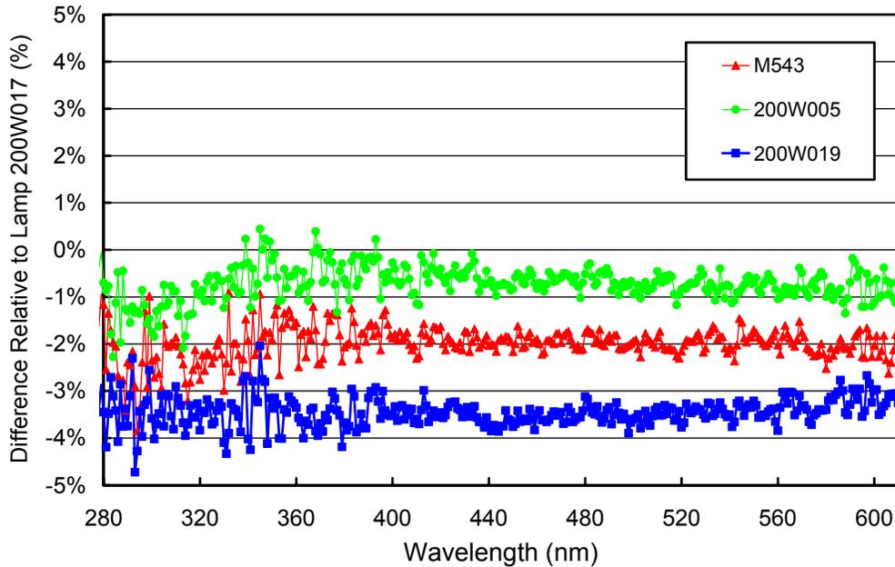
**Figure 5.1.2.** Comparison of McMurdo lamps M-543, 200W005, and 200W019 with the BSI traveling standard 200W017 at the beginning of the Volume 17 season (1/15/07).
