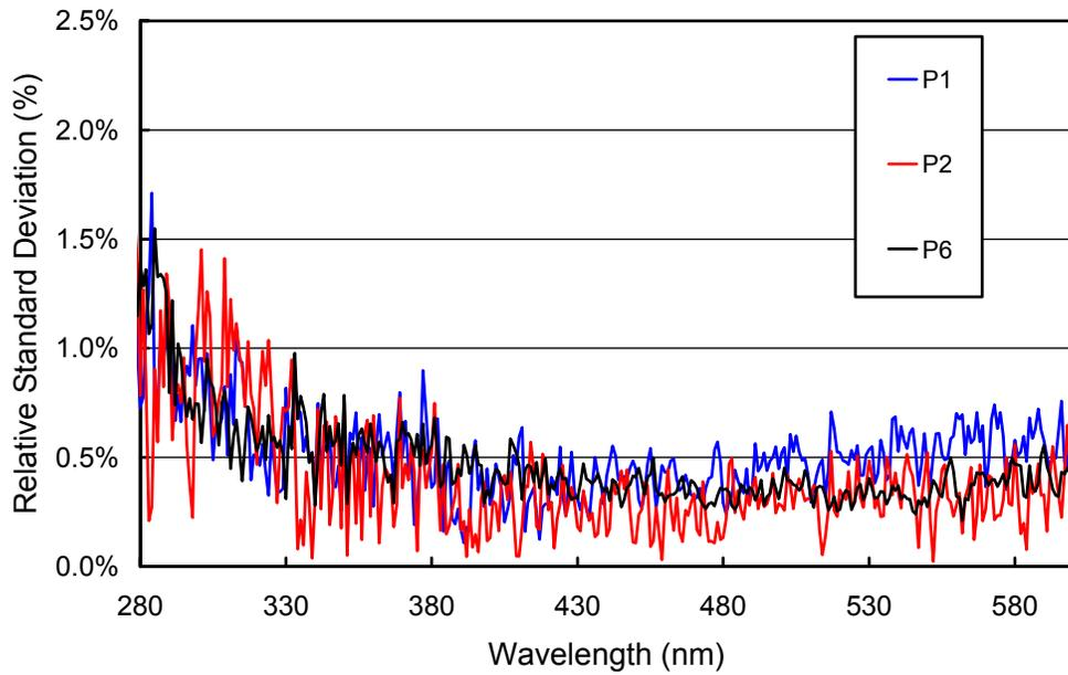
**Figure 5.1.5.** Ratio of standard deviation and average calculated from absolute calibration scans performed in Periods P1, P2, and P6.
