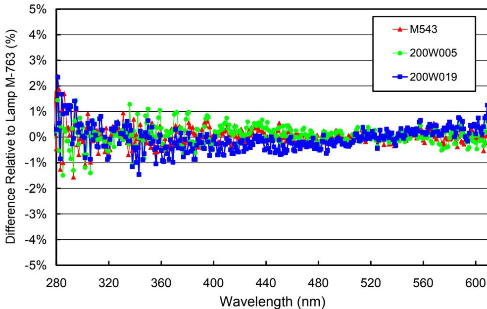
**Figure 5.1.1.** Comparison of McMurdo lamps M-543, 200W005, and 200W019 with the BSI traveling standard M-763 on 1/25/08. Lamp M-763 had been calibrated in June 2007 against four 1000-Watt FEL standards provided by CUCF and corrected for the misalignment in its holder.
