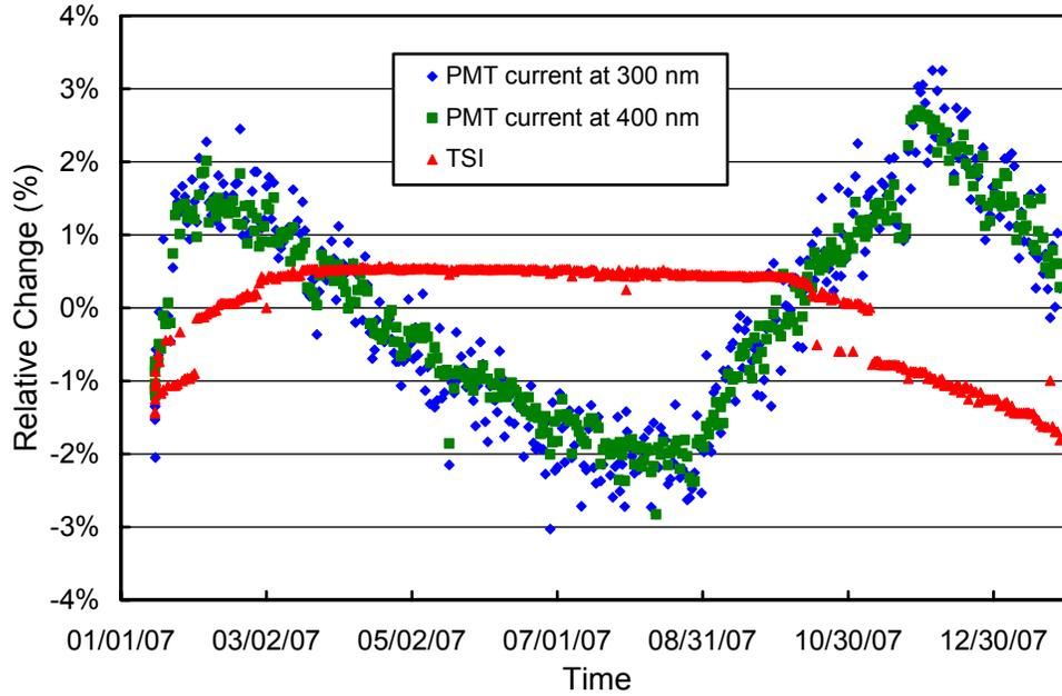
**Figure 5.1.3.** Time-series of PMT current at 300 and 400 nm, and TSI signal derived from measurements of the internal irradiance reference lamp during the McMurdo 2007/08 season. Data are normalized to the average value of the whole season.
