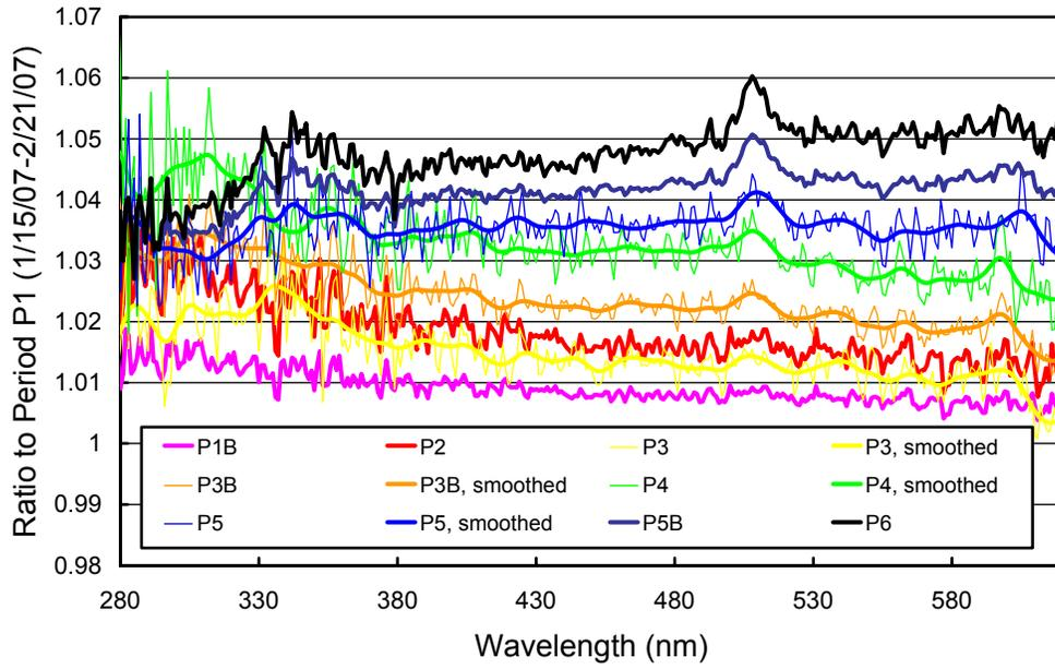
**Figure 5.1.4** Ratios of irradiance assigned to the internal reference lamp during periods P1B – P6, relative to Period P1.
