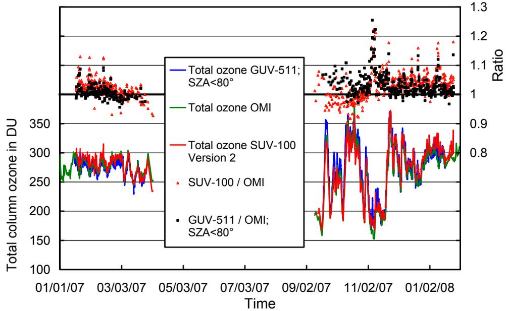
**Figure 5.1.11.** Comparison of total column ozone measurements from GUV-511, SUV-100 (Version 2 data), and OMI (v8.5, Collection 3). GUV-511 and SUV-100 measurements are plotted in 15 minute intervals. For calculating the ratio of both data sets, only GUV-511 measurements concurrent with OMI overpass data were evaluated. The cause of the spike observed in ratios GUV/OMI and SUV/OMI between 11/5/07 and 11/9/07 is unknown.
