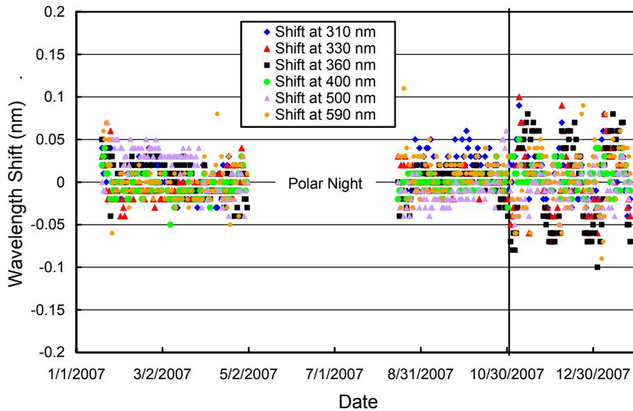
**Figure 5.1.8.** Check of the wavelength accuracy of final data at four wavelengths by means of Fraunhofer correlation. The noontime measurement has been evaluated for each day of the season. No correlation
