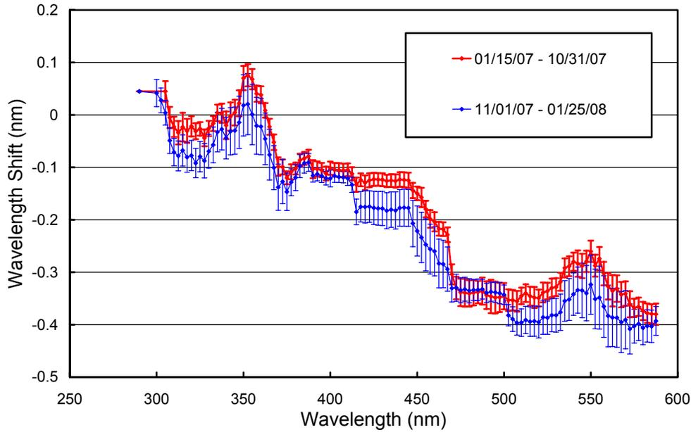
**Figure 5.1.7.** Monochromator non-linearity correction functions for McMurdo 2007/08 data. Error bars indicate the  $1\sigma$ -variation in each period.
