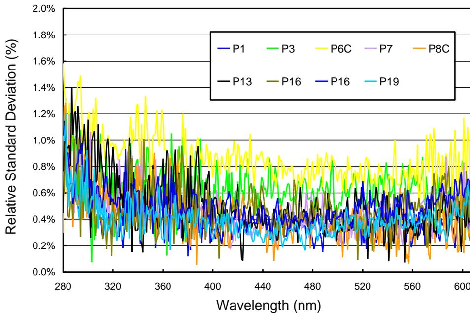
**Figure 5.2.6.** Relative standard deviation spectra for periods with more than two absolute scan.
