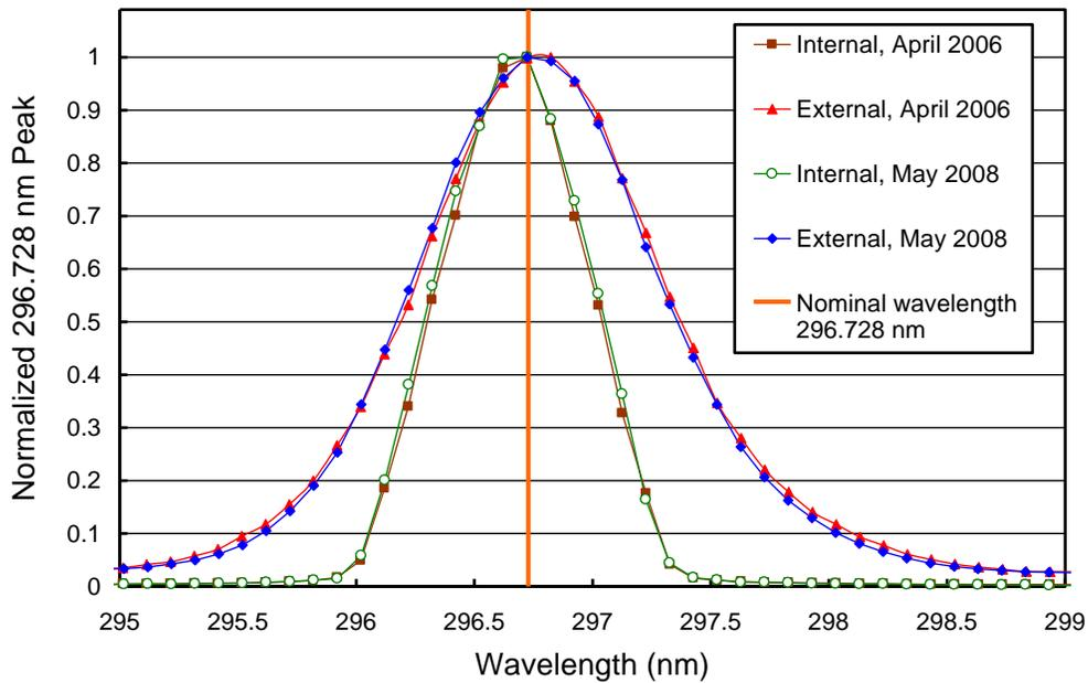
**Figure 5.2.10.** The 296.73 mercury line as registered by the PMT from external and internal sources. The wavelength scale is the same as that applied for solar measurements.
