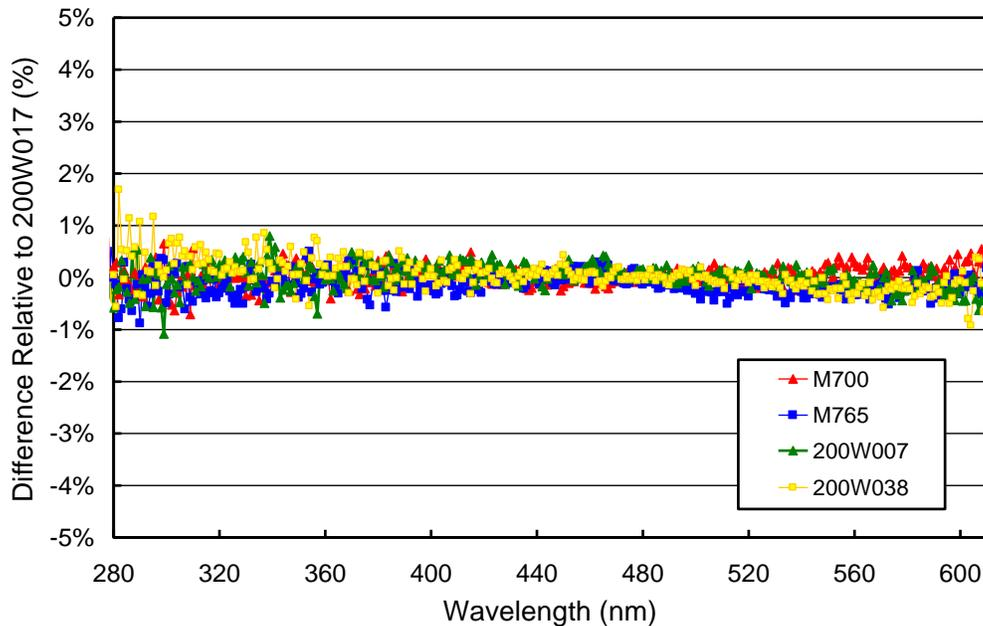
**Figure 5.2.2.** Comparison of Palmer lamps M-700, M-765, and 200W007 and lamp 200W038 with the BSI traveling standard 200W017 on 5/10/08. The calibrations of lamps 200W017 and 200W038 are traceable to the irradiance scale of four 1000-Watt FEL lamps calibrated by CUCF. Lamps M-700 and 200W007 were calibrated against the two traveling standards. The calibration of lamp M-765 is identical to that used at the beginning of the reporting period.
