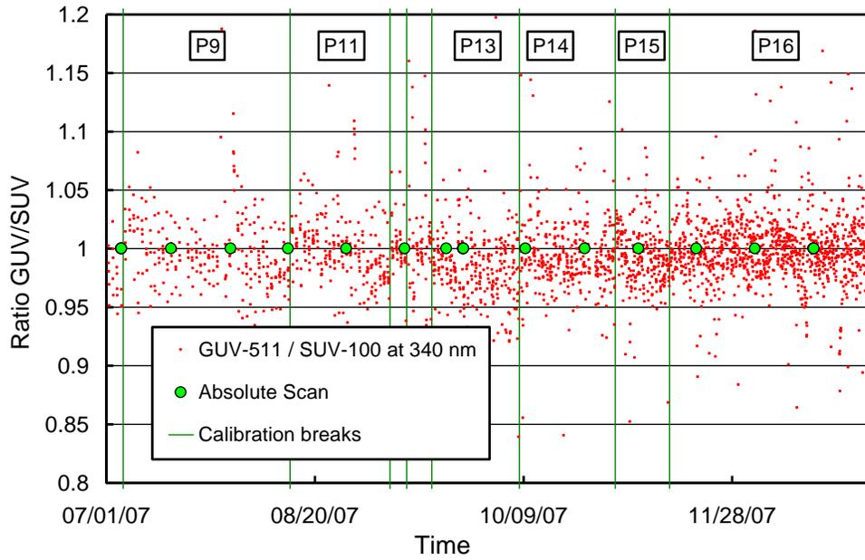
**Figure 5.2.5c.** Ratio of GUV-511 and SUV-100 measurements from the second half of 2007.
