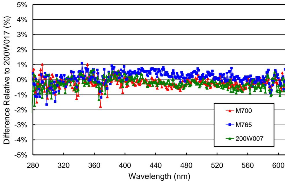
**Figure 5.2.1.** Comparison of Palmer lamps M-700, M-765, and 200W007 with the BSI traveling standard 200W017 on 4/28/06. The calibration of lamp 200W017 was established by Optronic Laboratories in March 2001.
