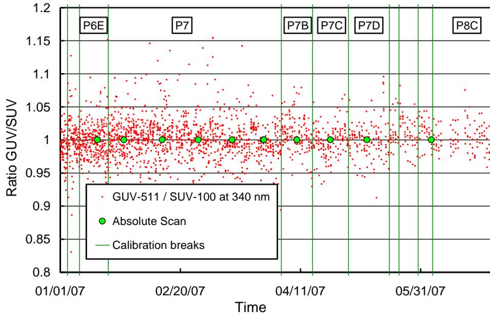
**Figure 5.2.5b.** Ratio of GUV-511 and SUV-100 measurements from the first half of 2007.
