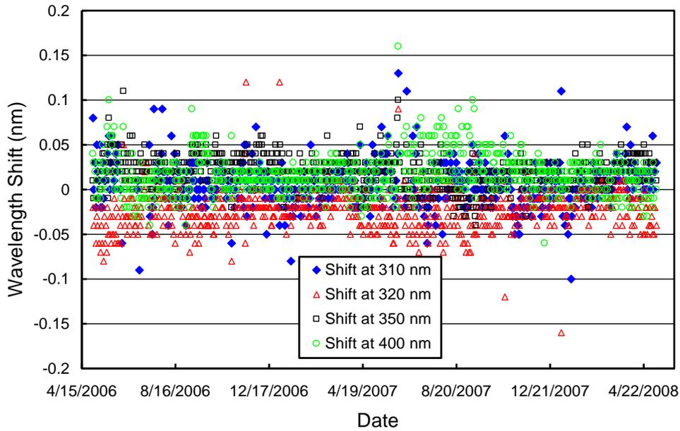
**Figure 5.2.9.** Wavelength accuracy check of the final data at four wavelengths by means of Fraunhofer-line correlation. Noontime measurements from every day of have been evaluated.
