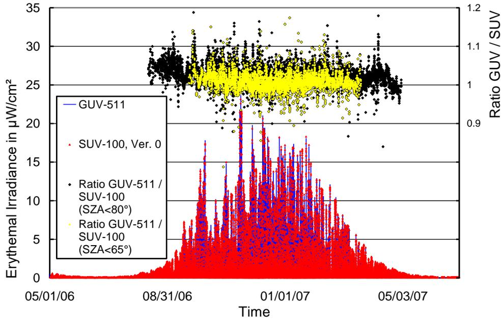
**Figure 5.2.11.** Comparison of erythemal irradiance measured by the SUV-100 spectroradiometer and the GUV-511 radiometer of the Volume 16 period. The ratio was filtered for measurements performed at solar zenith angles smaller than 80° (black markers) and 65° (yellow markers).
