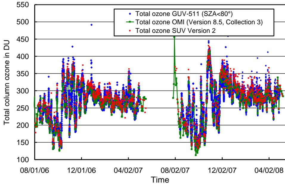
**Figure 5.2.13.** Comparison of total column ozone measurements from GUV-511, OMI, and SUV-100. GUV total ozone data are provided in 15 minute increments for solar zenith angles smaller than 80°. OMI data are from the “Version 8.4 Collection 3” data edition, which is approximately 2% smaller than the original OMI data release. SUV-100 data are from the “Version 2” data edition.
