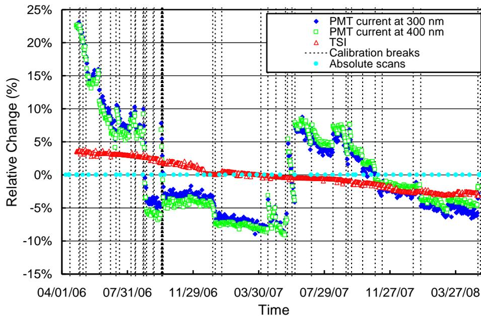
**Figure 5.2.3.** Time-series of PMT current at 300 and 400 nm, and TSI signal calculated from measurements of the internal irradiance reference lamp during the Palmer Volume 16 and 17 seasons. All data sets are normalized to their average values. Calibration breaks are indicated by vertical broken lines. Times of absolute scans are indicated by cyan circles.
