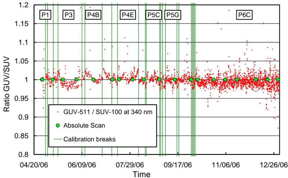
**Figure 5.2.5a.** Ratio of GUV-511 and SUV-100 measurements from 2006. Green lines indicate limits of calibration periods.
