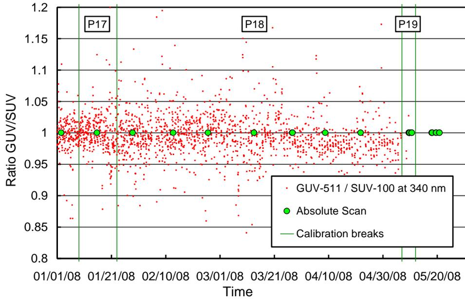
**Figure 5.2.5d.** Ratio of GUV-511 and SUV-100 measurements from 2008.
