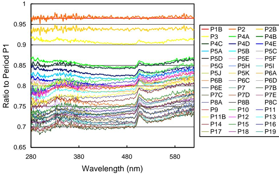
**Figure 5.2.4.** Ratios of spectral irradiance assigned to the internal reference lamp for periods P1B – P19, relative to Period P1. The large drift is caused by changes in the monochromator throughput.
