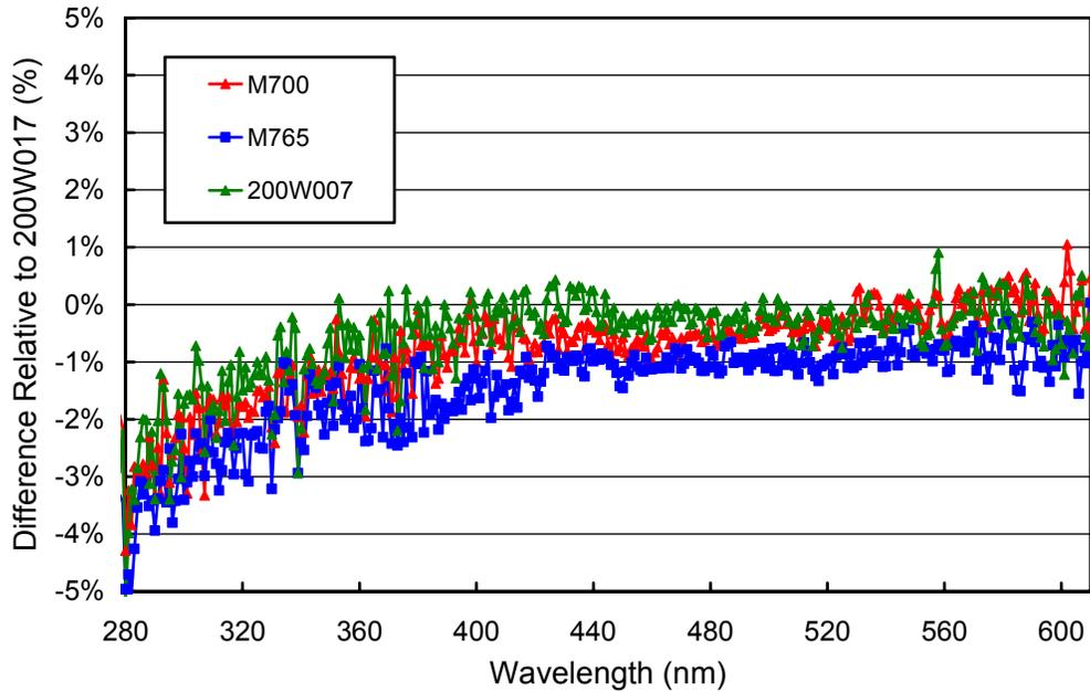
**Figure 5.2.1.** Comparison of Palmer lamps 200W007, M-700, and M-765 with the BSI traveling standard 200W017 on 4/14/06. Results are based on the calibrations of lamps 200W007, M-700, and M-765 used for Volumes 10 – 13.
