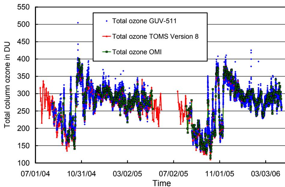
**Figure 5.2.12.** Comparison of total column ozone measurements from GUV-511, TOMS Earth Probe and OMI. GUV total ozone data are provided in 15 minute increments for solar zenith angles smaller than 80°.
