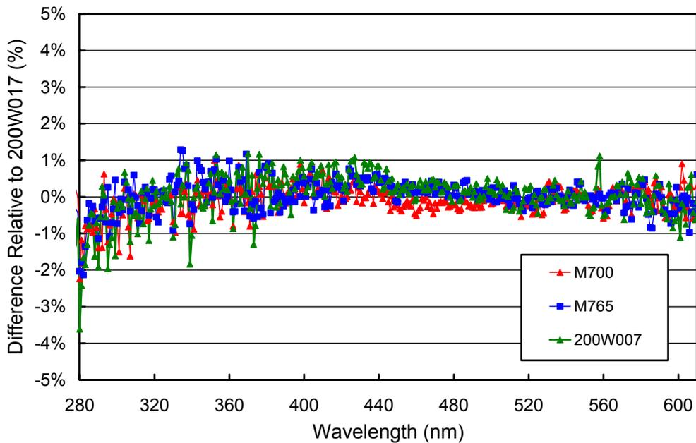
**Figure 5.2.2.** Comparison of Palmer lamps 200W007, M-700, and M-765 with the BSI traveling standard 200W017 on 4/14/06. Results are based on the updated calibration functions of lamps 200W007, M-700, and M-765 that were established following the 2006 site visit. These calibration functions were used for processing of solar data of the reporting period.
