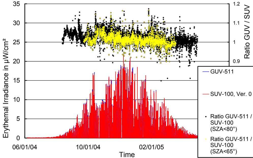
**Figure 5.2.10.** Comparison of erythemal irradiance measured by the SUV-100 spectroradiometer and the GUV-511 radiometer of the Volume 14 period. The ratio was filtered for measurements performed at solar zenith angles smaller than 80° (black markers) and 65° (yellow markers).
