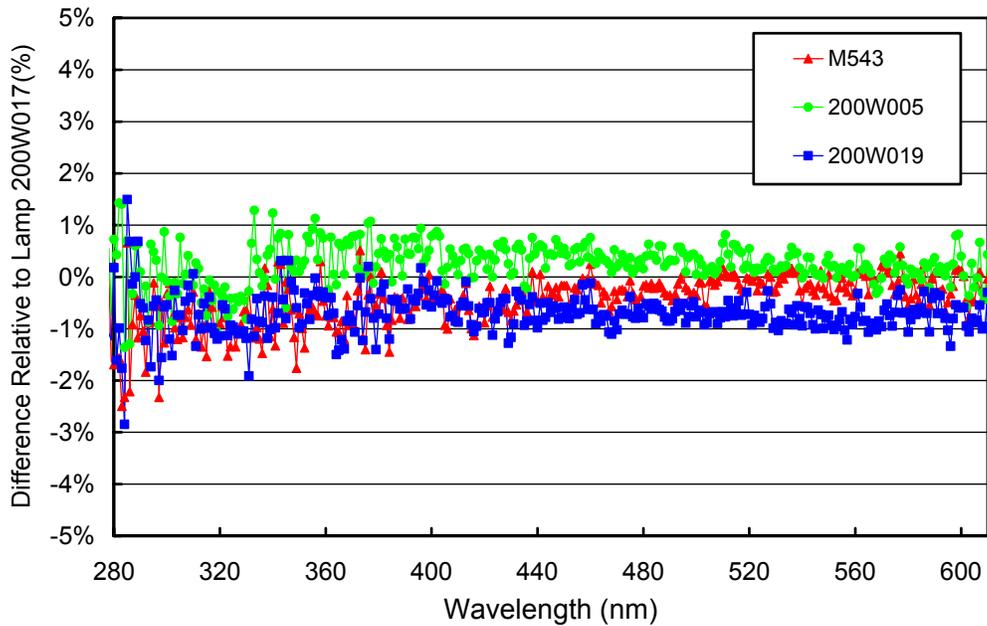
**Figure 5.1.2.** Comparison of McMurdo lamps M-543, 200W005, and 200W019 with the BSI traveling standard 200W017 at the end of the season (1/20/06). The new calibration of lamp 200W005 was used.
