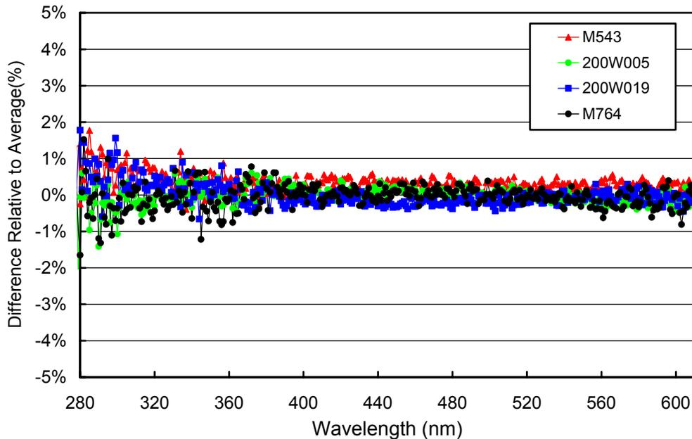
**Figure 5.1.1.** Comparison of McMurdo lamps M-543, 200W005, and 200W019 and the BSI traveling standard M-764 at the beginning of the season (1/28/05). The 2002 calibration of lamp 200W005 was used.
