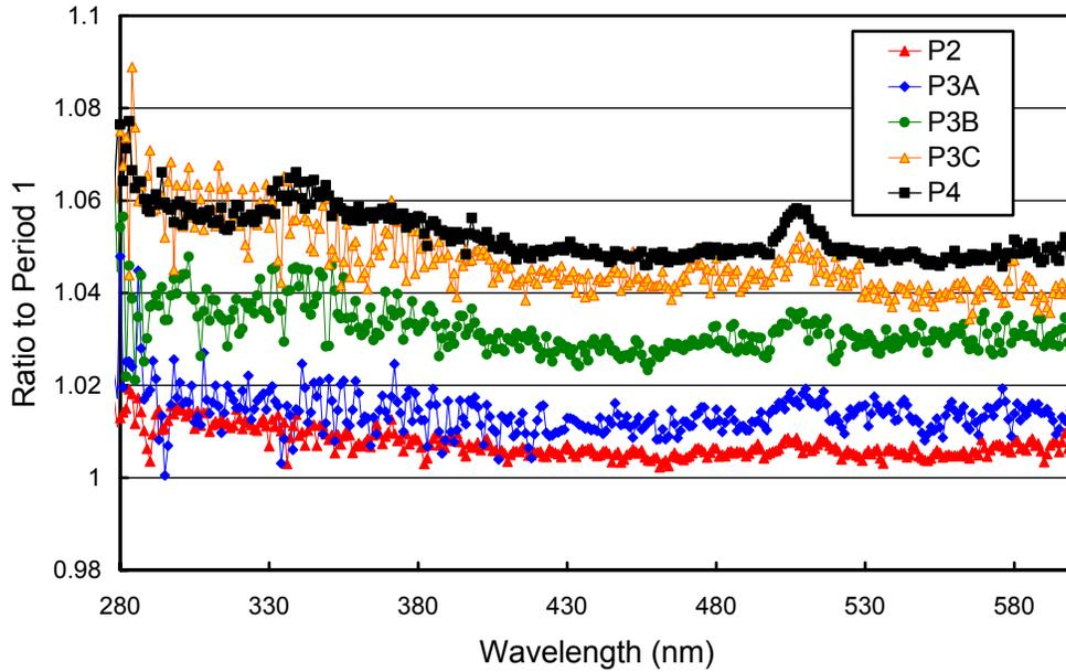
**Figure 5.1.4** Ratio of irradiance assigned to the internal reference lamp relative to Period P1 (01/27/05 - 6/30/05).
