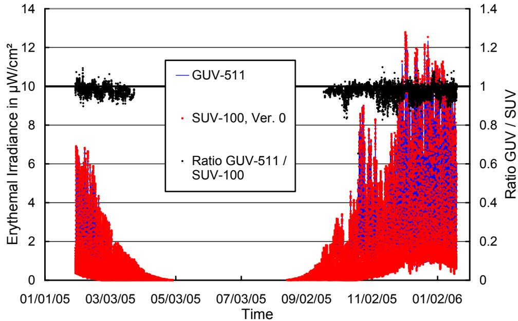
**Figure 5.1.10.** Comparison of erythemal irradiance measured by the SUV-100 spectroradiometer and the GUV-511 radiometer. All data are based on “Version 0” (cosine-error uncorrected) data.
