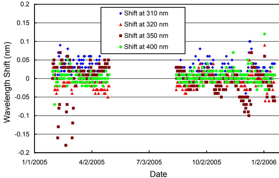
**Figure 5.1.8.** Check of the wavelength accuracy of final data at four wavelengths by means of Fraunhofer correlation. The noontime measurement has been evaluated for each day of the season. No correlation data is available during Polar Night.
