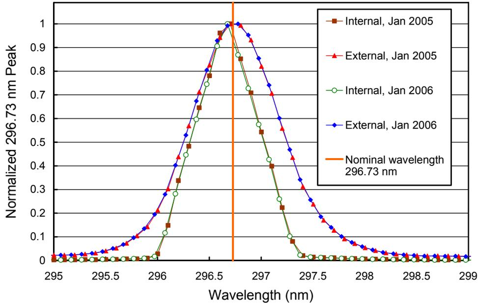
**Figure 5.1.9** The 296.73 mercury line as registered by the PMT from external and internal sources. The wavelength scale is the same as applied for solar measurements. It is assumed that the wavelength registration of the monochromator did not shift between internal and external scans, which were close in time.
