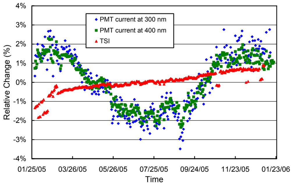
**Figure 5.1.3.** Time-series of PMT current at 300 and 400 nm, and TSI signal derived from measurements of the internal irradiance reference lamp during the McMurdo 2005/06 season. The data is normalized to the average value of the whole season.
