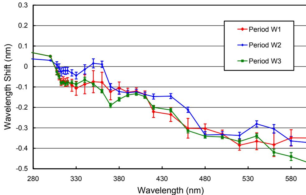
**Figure 5.1.7.** Monochromator non-linearity correction functions for McMurdo 2005/06 data. The error bars indicate the  $1\sigma$ -variation in each period.
