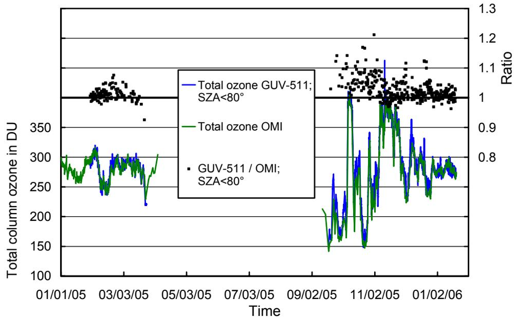
**Figure 5.1.11.** Comparison of total column ozone measurements from GUV-511 and OMI. GUV-511 measurements are plotted in 15 minute intervals. For calculating the ratio of both data sets, only GUV-511 measurements concurrent with OMI overpass data were evaluated.
