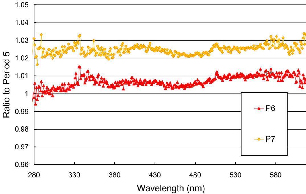
**Figure 5.2.5.** Ratios of irradiance spectra assigned to the Internal Lamp #2 in Periods P6 and P7 compared to Period P5.
