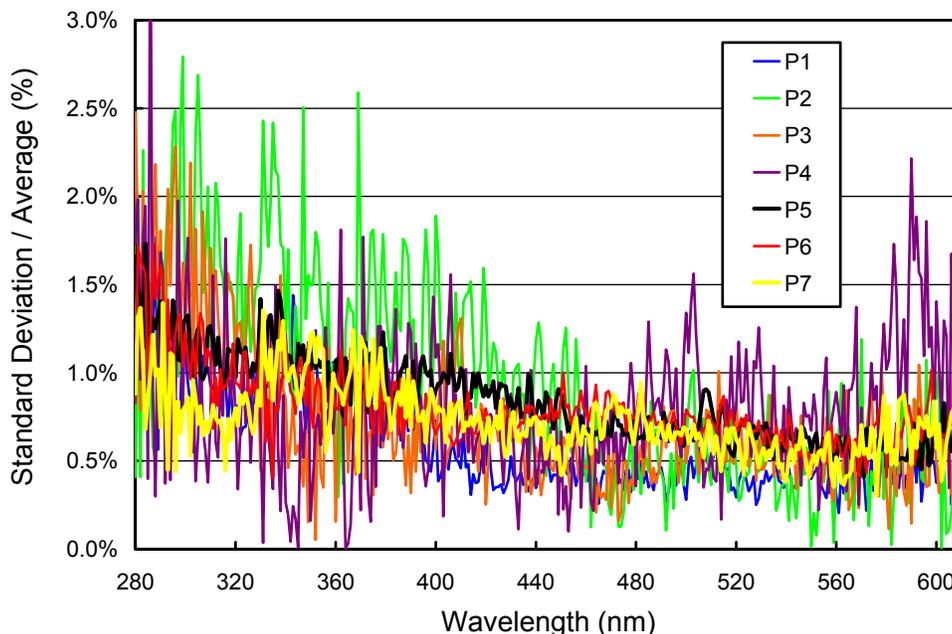
Figure 5.2.6. Ratio of standard deviation and average calculated from the absolute calibration scans.
