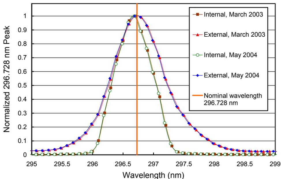
**Figure 5.2.10.** The 296.73 mercury line as registered by the PMT from external and internal sources. The wavelength scale is the same as applied for solar measurements.
