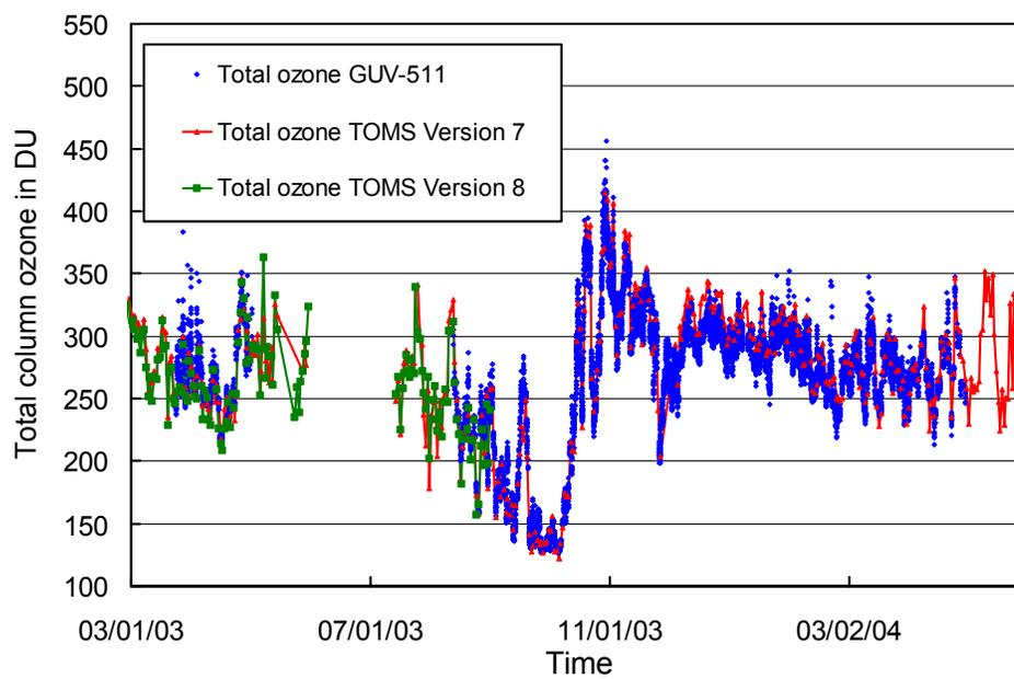
**Figure 5.2.12.** Comparison of total column ozone measurements from GUV-511, and NASA/TOMS Earth Probe satellite.
