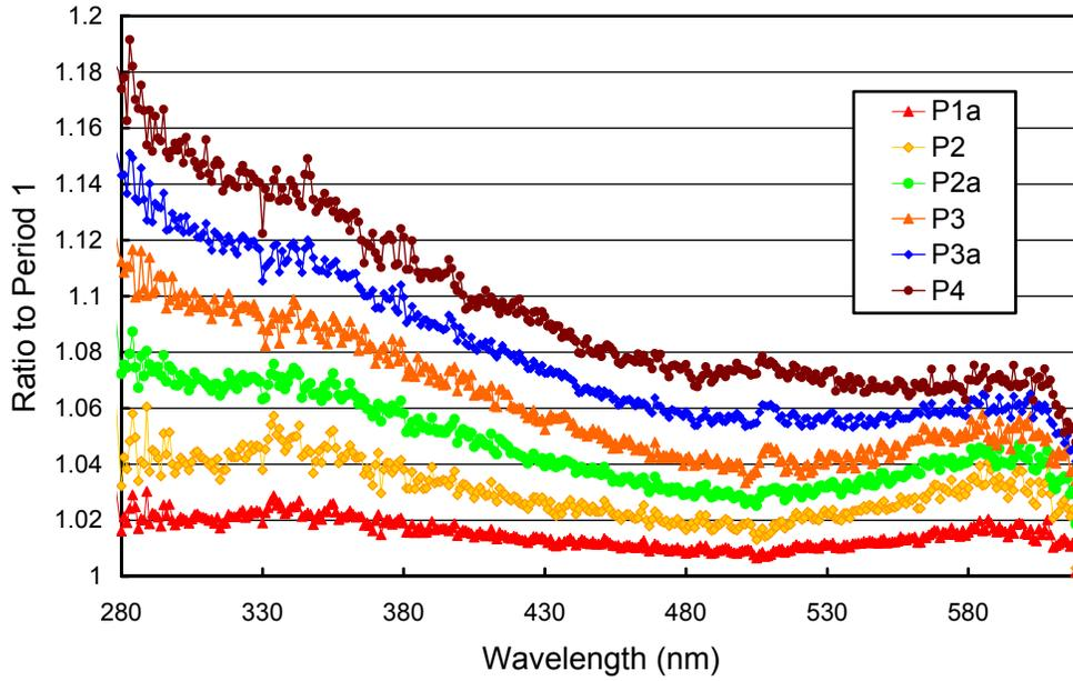
**Figure 5.2.4.** Ratios of irradiance spectra assigned to the Internal Lamp #1 in Periods P1a – P4 relative to Period P1.
