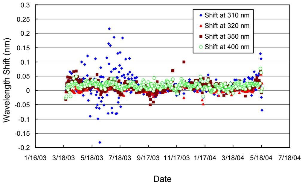
Figure 5.2.9. Wavelength accuracy check of the final data at four wavelengths by means of Fraunhofer correlation. The noontime measurement has been evaluated for each day of the season.
