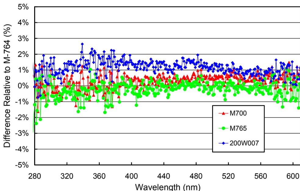
**Figure 5.2.2.** Comparison of Palmer lamps 200W007, M-700, and M-765 with the BSI traveling standard M-764 at the end of the season (5/20/04).
