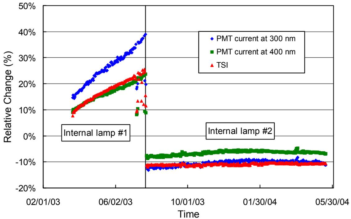
**Figure 5.2.3.** Time-series of PMT current at 300 and 400 nm, and TSI signal during measurements of the internal lamp during the Palmer 2003/04 season. Internal lamp #1 exhibited a larger drift, became unstable on 7/1/03, and was replaced on 7/23/03. The data is normalized to the average of all periods.
