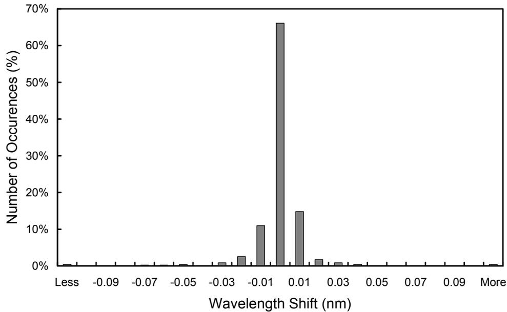
**Figure 5.2.7.** Differences in the measured position of the 296.73 nm mercury line between consecutive wavelength scans. The x-labels give the center wavelength shift for each column. Thus the 0-nm histogram column covers the range -0.005 to +0.005 nm. “Less” means shifts smaller than -0.105 nm; “more” means shifts larger than 0.105 nm.
