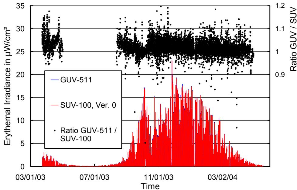
**Figure 5.2.11.** Comparison of erythemal irradiance measured by the SUV-100 spectroradiometer and the GUV-511 radiometer. All data are based on "Version 0," see text. The ratio is restricted to measurements at SZAs smaller than  $80^\circ$ .
