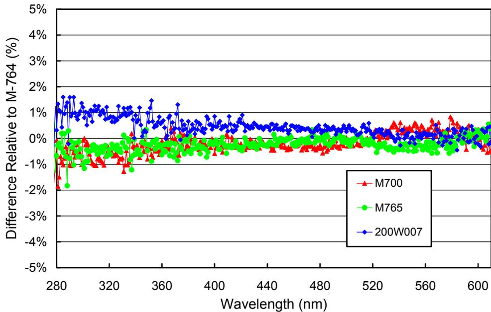
**Figure 5.2.1.** Comparison of Palmer lamps 200W007, M-700, and M-765 with the BSI traveling standard M-764 at the beginning of the season (3/22/03).
