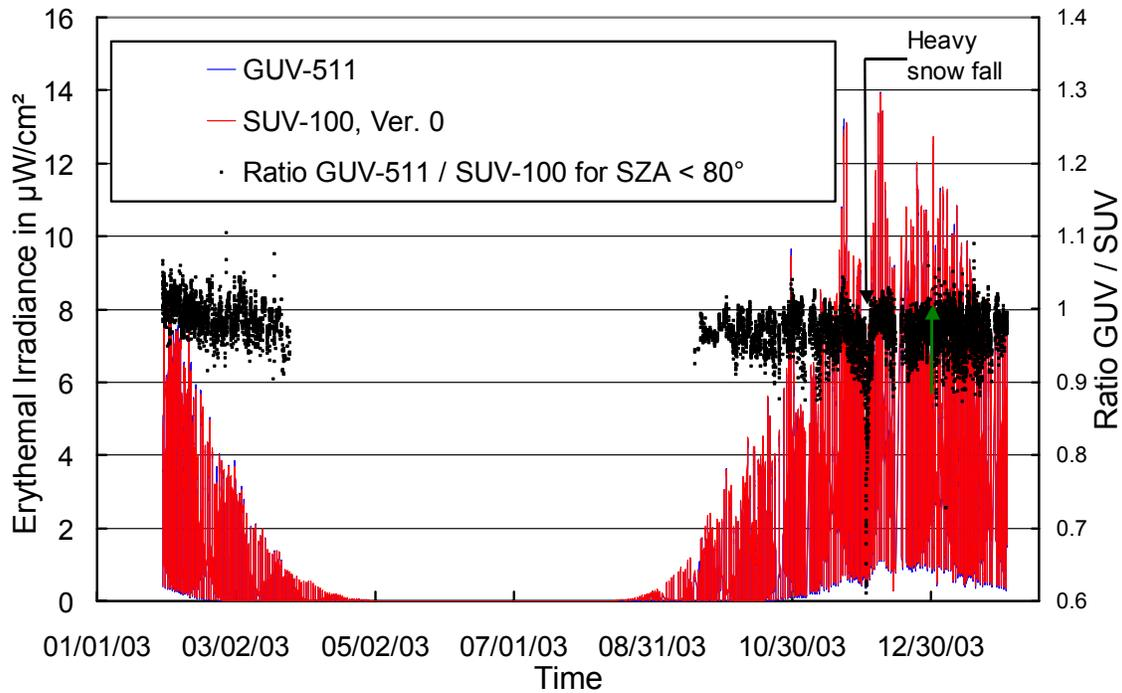
**Figure 5.1.10.** Comparison of erythemal irradiance measured by the SUV-100 spectroradiometer and the GUV-511 radiometer. All data is based on “Version 0” (cosine-error uncorrected) data, see text.
