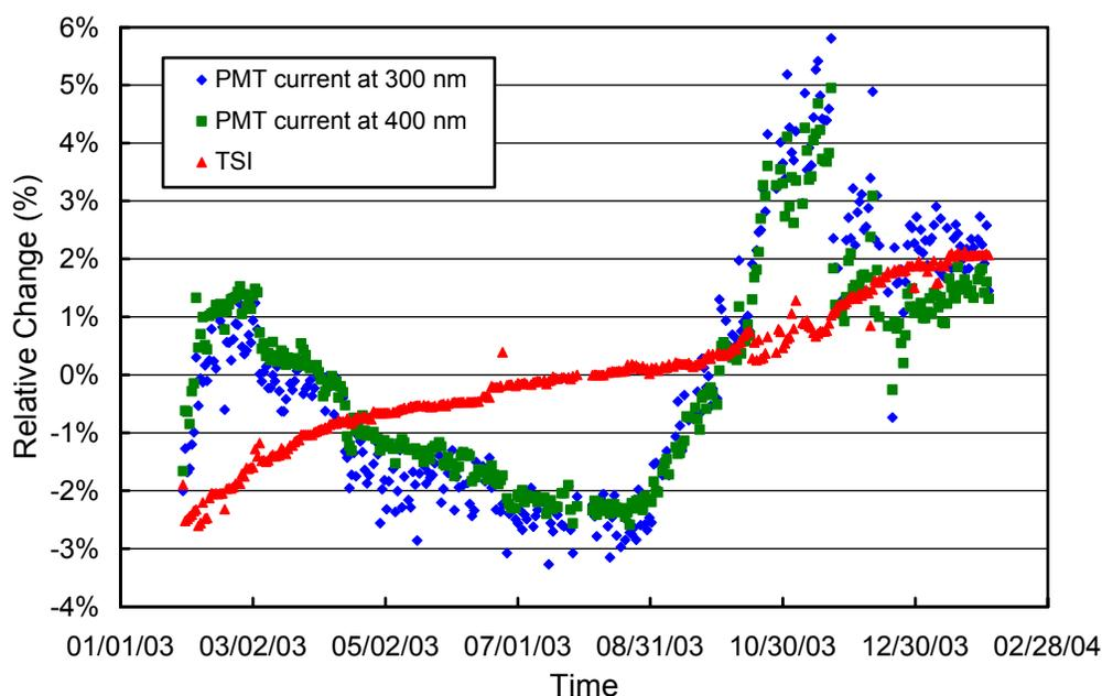
**Figure 5.1.3.** Time-series of PMT current at 300 and 400 nm, and TSI signal during measurements of the internal irradiance reference lamp during the McMurdo 2003/04 season. The data is normalized to the average value of the whole season.
