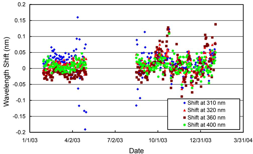
**Figure 5.1.8.** Check of the wavelength accuracy of the final data at four wavelengths by means of Fraunhofer correlation. The noontime measurement has been evaluated for each day of the season. No correlation data is available during the polar night.
