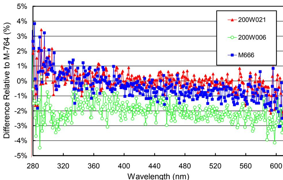
**Figure 5.3.2.** Comparison of South Pole lamps 200W006, 200W021, M-666 with the BSI traveling standard M-764 at the end of the season on 1/13/02.
