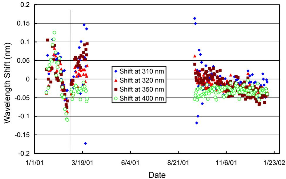
**Figure 5.3.8.** Wavelength accuracy check of the final data at four wavelengths by means of Fraunhofer correlation. The noontime measurement has been evaluated for each day of the season. No data exist during polar night.
