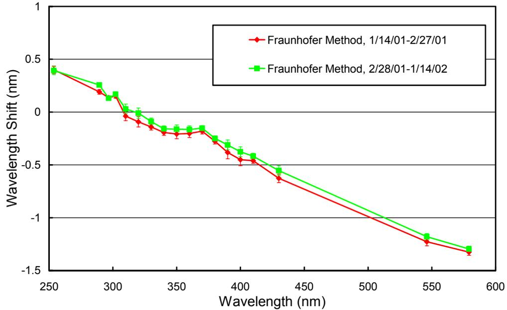
**Figure 5.3.7.** Monochromator non-linearity functions for the South Pole 2001/02 season. The error bars show the  $1\sigma$  standard deviation of the wavelength shifts.
