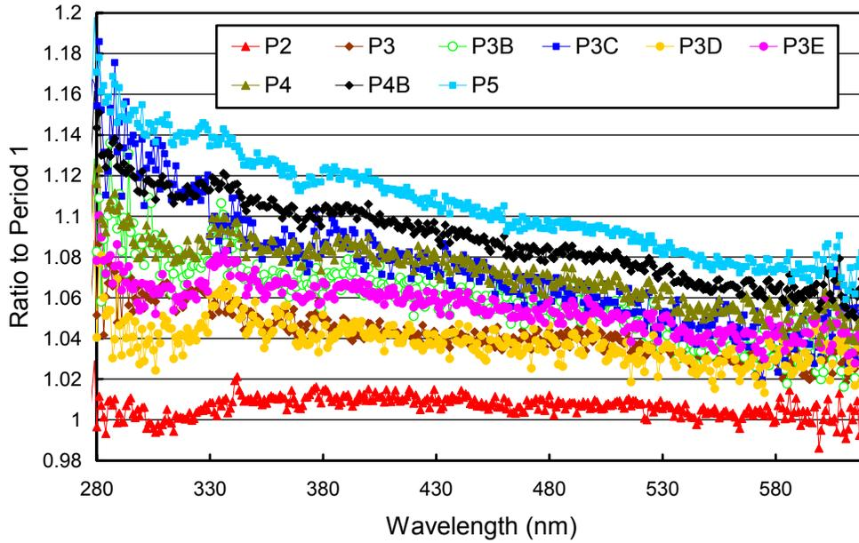
Figure 5.3.4. Ratios of the irradiance assigned to the internal lamp relative to Period 1.
