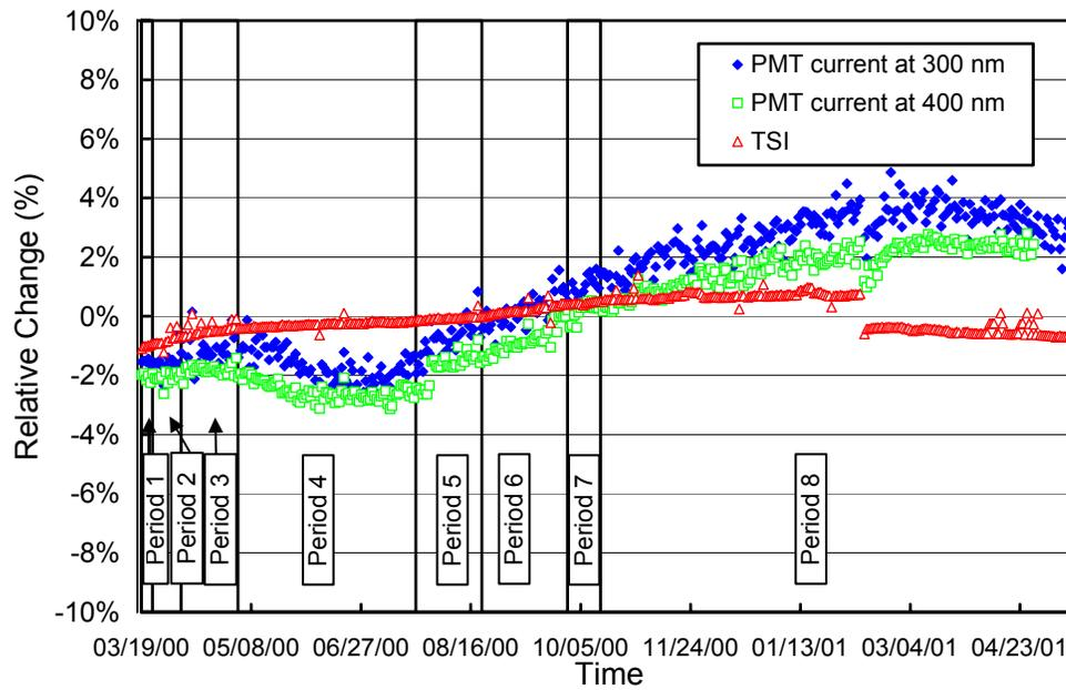
**Figure 5.2.3.** Time-series of PMT current at 300 and 400 nm, and TSI signal during measurements of the response lamp during the Palmer 2000/01 season. The data is normalized to the average of all periods.
