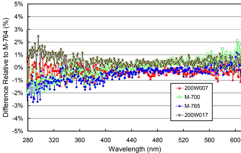
**Figure 5.2.2.** Comparison of Palmer lamps 200W007, M-700, and M-765 with the BSI traveling standard M-764 at the end of the season (5/18/01 - 5/24/01).
