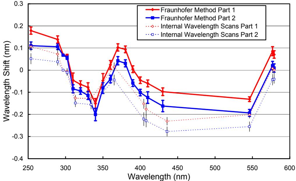
**Figure 5.2.7.** Monochromator non-linearity for the Palmer 2000/01 season. Thick lines: Correction function calculated with the Fraunhofer-correlation method, and applied to correct the Palmer Volume 10 data. Part one includes the period 3/19/00 – 11/1/00; Part 2 the remainder of the season. Thin broken lines: Correction function calculated with the method that was historically applied. The error bars show the  $1\sigma$  standard deviation of the wavelength shifts.
