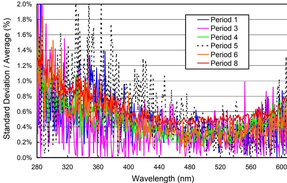
**Figure 5.2.5.** Ratio of standard deviation and average calculated from the absolute calibration scans. The data for Periods 2 and 7 are not shown since they are based on one scan only.
