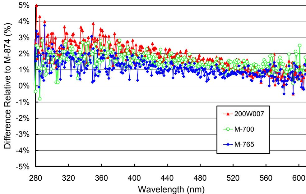
**Figure 5.2.1.** Comparison of Palmer lamps 200W007, M-700, and M-765 with the BSI traveling standard M-874 at the beginning of the season.
