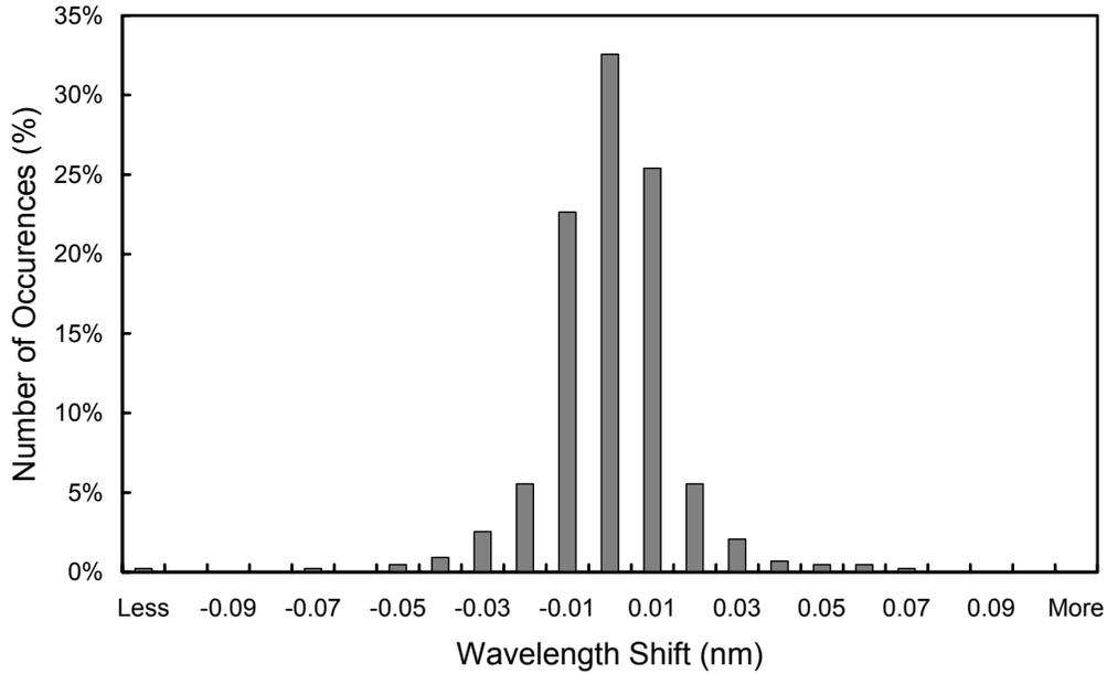
**Figure 5.2.6.** Differences in the measured position of the 296.73 nm mercury line between consecutive wavelength scans. The x-labels give the center wavelength shift for each column. Thus the 0-nm histogram column covers the range -0.005 to +0.005 nm. “Less” means shifts smaller than -0.105 nm; “more” means shifts larger than 0.105 nm.
