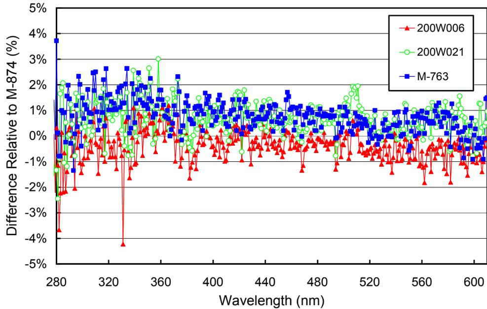
**Figure 5.3.1.** Comparison of South Pole lamps 200W006, 200W021, and M-763 with the BSI traveling standard M-874 at the start of the season on 1/15/99.
