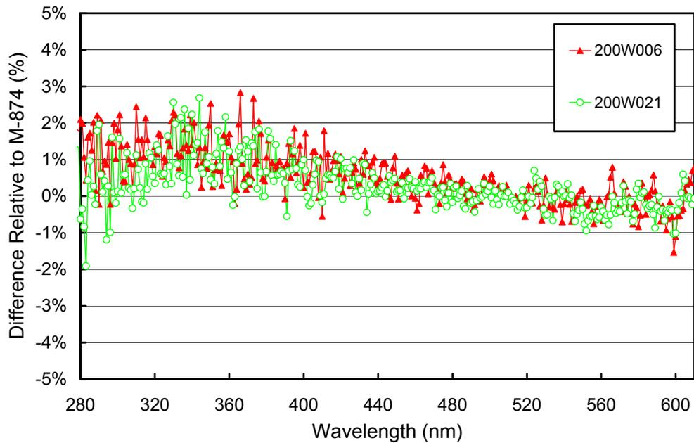
**Figure 5.3.2.** Comparison of South Pole lamps 200W006, and 200W021 with the BSI traveling standard M-874 at the end of the season on 1/18/00.
