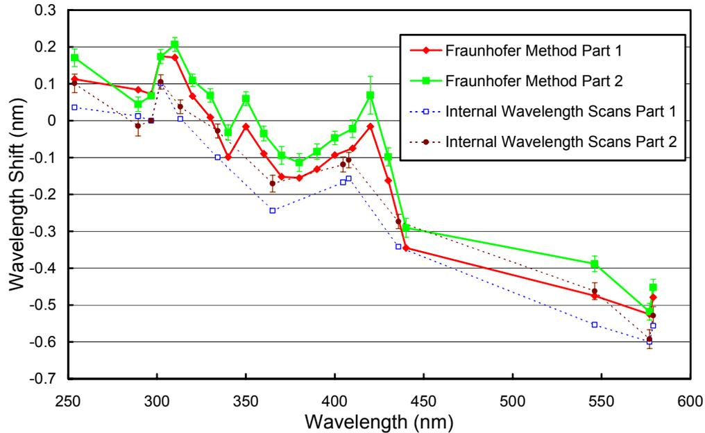
**Figure 5.3.7.** Monochromator non-linearity for the South Pole 1999-2000 season. Thick lines: Correction functions calculated with the Fraunhofer-correlation method, applied to correct the South Pole Volume 9 data. Thin broken lines: Correction function calculated with the method that was historically applied. The offset difference between both methods is 0.07 nm. The error bars show the  $1\sigma$  standard deviation of the wavelength shifts.
