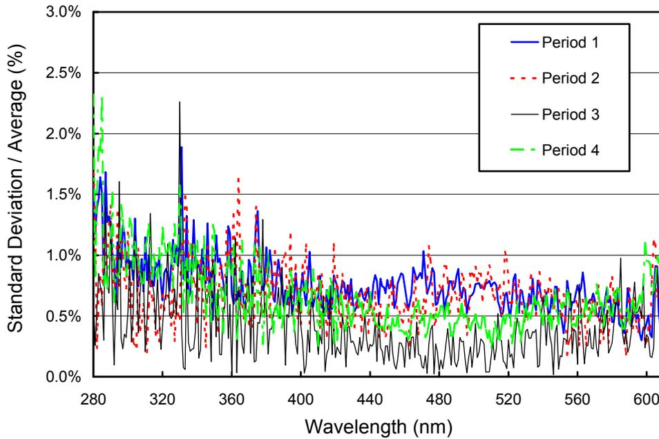
**Figure 5.3.5.** Ratio of standard deviation and average calculated from the absolute calibration scans measured during the South Pole 1999-2000 season.
