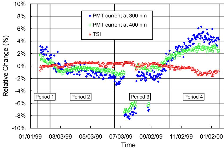
**Figure 5.3.3.** Time-series of PMT current at 300 and 400 nm, and TSI signal during measurements of the internal irradiance standard performed during the South Pole 1999-2000 season. The data are normalized to the average of the whole period. The two low clusters of points in Period 3 were during the polar night.
