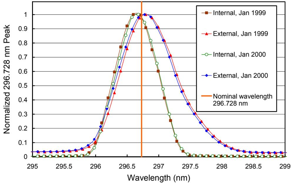
**Figure 5.3.9.** The 296.73 mercury line as registered by the PMT from external and internal sources. The wavelength scale is the same as applied for solar measurements, i.e., it is based on a combination of internal scans and the Fraunhofer-correlation method.
