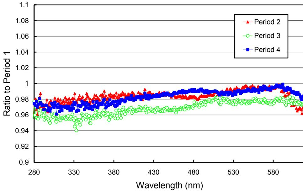
**Figure 5.3.4.** Ratios of the irradiance assigned to the internal lamp in Periods 2 – 4, relative to Period 1.
