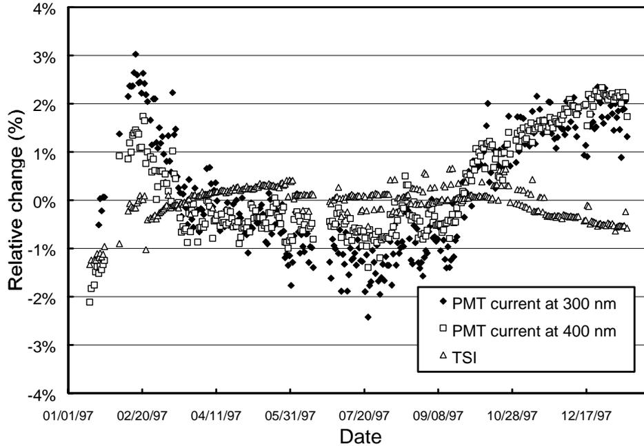
**Figure 5.2.12.** Time-series of PMT current at 300 and 400 nm and TSI signal during measurements of the response lamp in the whole McMurdo 1997/98 season. The data is normalized to the average of the whole season.
