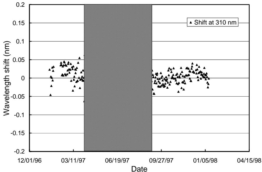
**Figure 5.2.10.** Check of the wavelength accuracy of the final data by means of Fraunhofer correlation. For each day of the season the noontime measurement at 310 nm has been evaluated. Outside the shaded
