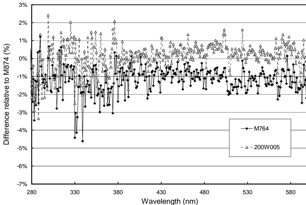
**Figure 5.2.15.** Result of season closing calibrations McMurdo, 1/14/98: Comparison of McMurdo lamps M-764 and 200W005 with the traveling standard M-874.
