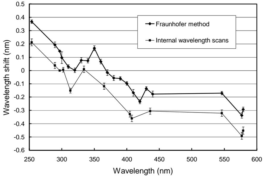
**Figure 5.2.9.** Functions expressing the monochromator non-linearity for McMurdo. Thick line: Function calculated with the Fraunhofer-correlation method. This function was applied to correct the McMurdo Volume 7 data. Thin line: Function calculated with the method that was historically applied. The offset between both methods is 0.146 nm. Both functions represent average wavelength shifts for the 1997/98 season. The error bars give the  $1\sigma$  standard deviation of the wavelength shifts.
