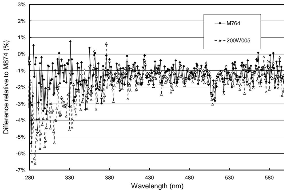
**Figure 5.2.14.** Result of season opening calibrations, McMurdo, 2/4/97: Comparison of McMurdo lamps M-764 and 200W005 with the traveling standard M-874.
