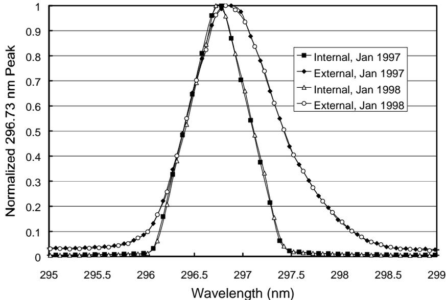
**Figure 5.2.11.** The 296.73 mercury spectral line as registered by the PMT from external and internal source.
