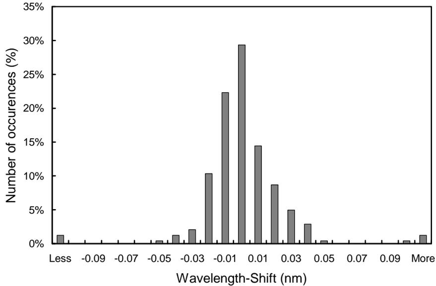
**Figure 5.2.8.** Differences in the measured position of the 296.73 nm Mercury line between consecutive wavelength scans. The x-labels give the center wavelength shift for each column. Thus the 0-nm histogram column covers the range -0.005 to +0.005 nm. “Less” means shifts smaller than -0.105 nm; “more” means shifts larger than 0.105 nm.
