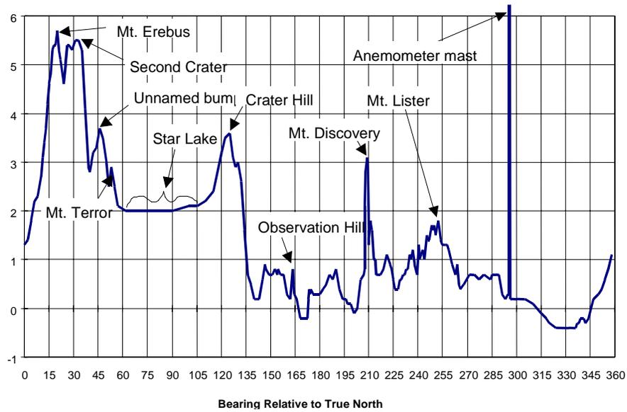
**Figure 5.2.2.** This chart displays the obstructions in the collector's field-of-view at Arrival Heights. Units are in degrees above the horizon vs. bearing relative to True North.
