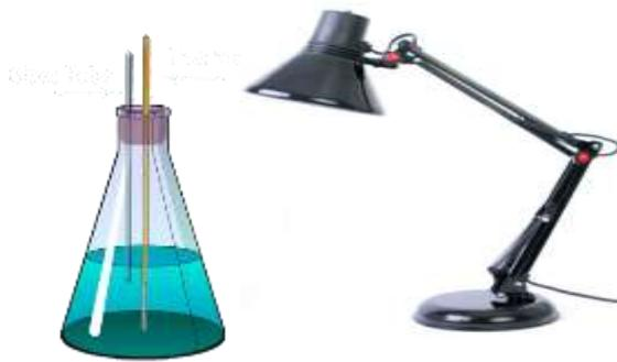
3. Have a student report the temperature of the water and mark the water level in the glass tube with marker or piece of tape.
