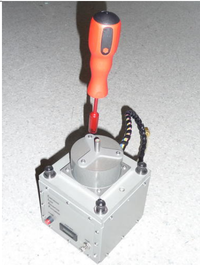
Top view of CLAP with top secured. To open CLAP for filter replacement unscrew the four nuts on top using the torque driver.
